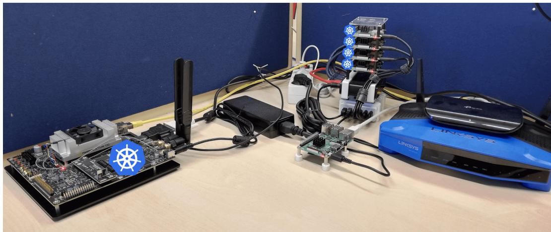
Figure 4.3: Picture of the testbed's edge nodes and their network devices
