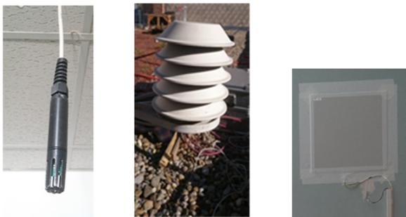
Fig. 7. Left: The Lin Picco sensor inside (protected by a plastic cover). Middle: Lin Picco sensor exterior protected by protective shield. Right: Heat flux film.
