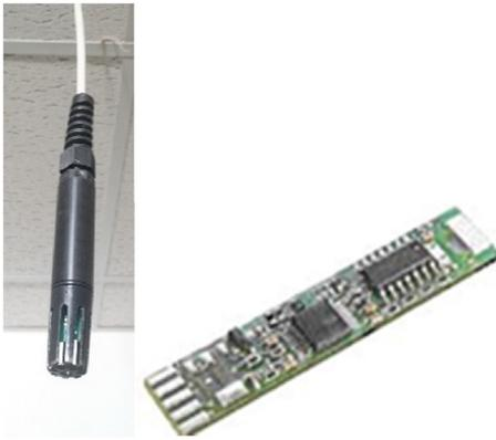
**Fig. 4.** Lin Picco A05. Left: With protective cover. Right: The chip without the protective cover.
