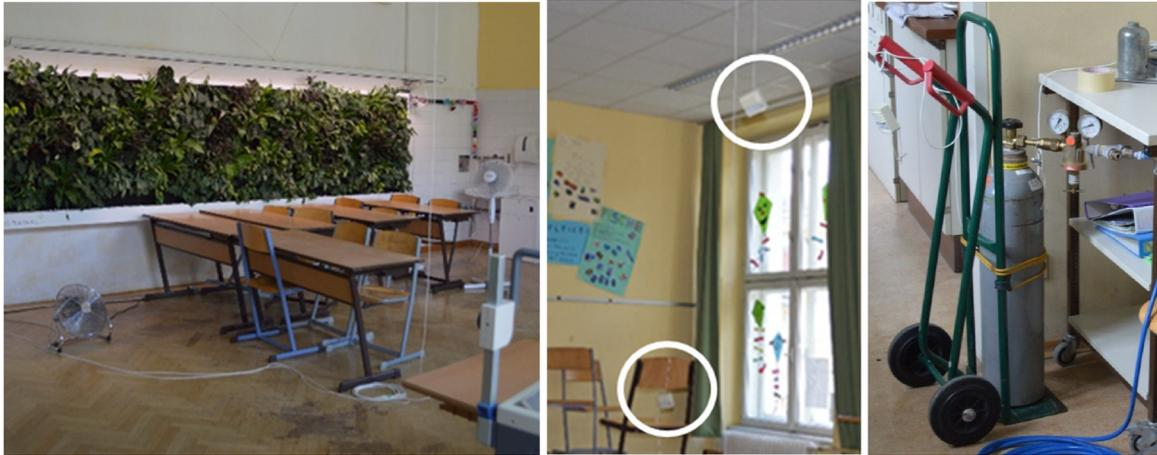
Fig. 10. Left: Fans in the classroom to distribute the CO<sub>2</sub> equally in the room. Middle: CO<sub>2</sub>-sensors in two different heights. Right: CO<sub>2</sub>-pressure cylinder.
