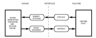
Figure 2.1: Interdependency between human and machine. The human interacts with the machine through an interface [62].
