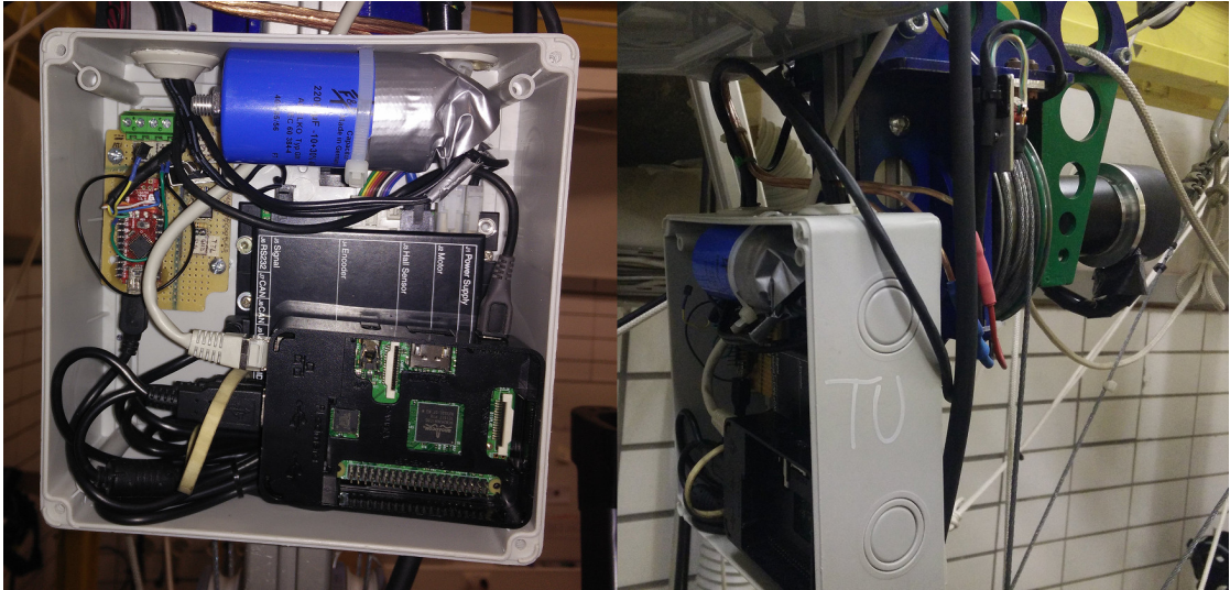
Figure 4.8: The EPOS controller device. The left-hand side image shows the controller, with the Arduino Nano (top left), and the Maxon Motors EPOS2 24/5 Digital positioning controller and the Raspberry Pi (bottom right). The blue cylinder at the top right is a capacitor needed to smooth out voltage spikes coming from the power supply. The right-hand side image depicts the controller including (from left to right) the clutch and the servo motor.
