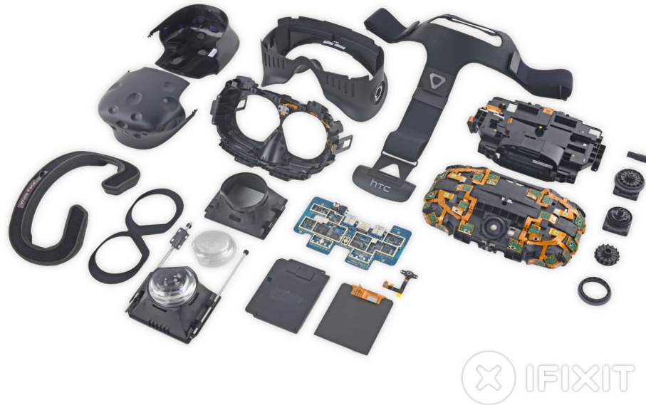
Figure 2.3: The HTC Vive uses lenses (bottom row, center) to project the image creating device further away from the user's eye. The housings of these lenses are mounted onto a mechanic which allows to move their position on the left-and-right axis. This enables the device to adapt to different eye spacings. Both approaches were described in Heilig's patent in 1957.
