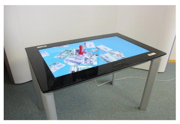
Figure 2.18: The "Fotokiste" prototype illustrating a tangible object shaped as a red punch that triggers the visualization of privately shared pictures.
