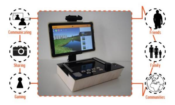
Figure 2.17: *KithNKin* prototype illustrating a standard tablet and a hardware platform for the tangible interaction [Con18a].
