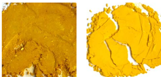
(a) \text{BiVO}_4 powder without microwave irradiation (b) \text{BiVO}_4 powder with microwave irradiation
