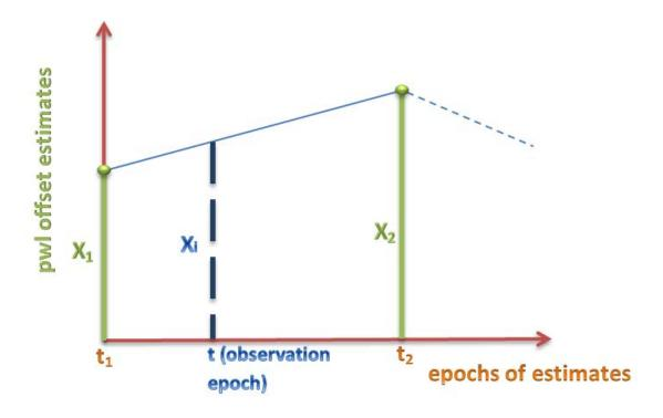
Figure 2.2.: Continuous piece-wise linear offsets (CPWLO).
