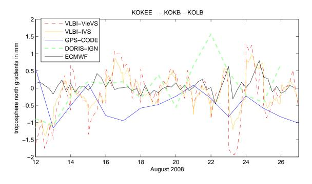
Figure A.7.2.: Troposphere north gradients at co-located site Kokee in USA during IVS-CONT08.
