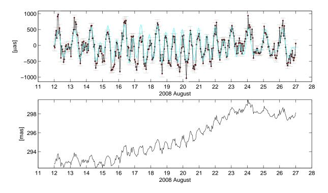
Figure 8.13.: In the upper figure, grey bars show the VieVS hourly (at UTC integer hours) CPWLO  $dx_p$  estimates with their formal errors during IVS-CONT08. The total hourly  $\Delta x$  values of the HF-ERP models are shown in the same plot in cyan. In the lower plot, linearly interpolated  $(x_p)_{IERS}$  plus VieVS hourly CPWLO  $dx_p$  estimates are shown. The VieVS analysis options are given in Tables 8.2 and 8.4.
