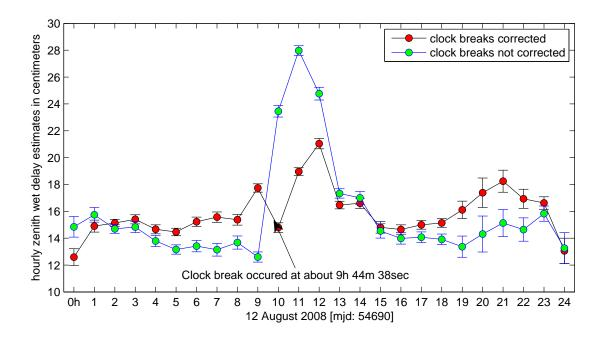
Figure 4.7.: CPWLO of hourly ZWD estimates of Zelenchukskaya VLBI antenna during the session 08AUG12XA, with and without  $\sim 60$  cm clock break at Zelenchukskaya corrected.
