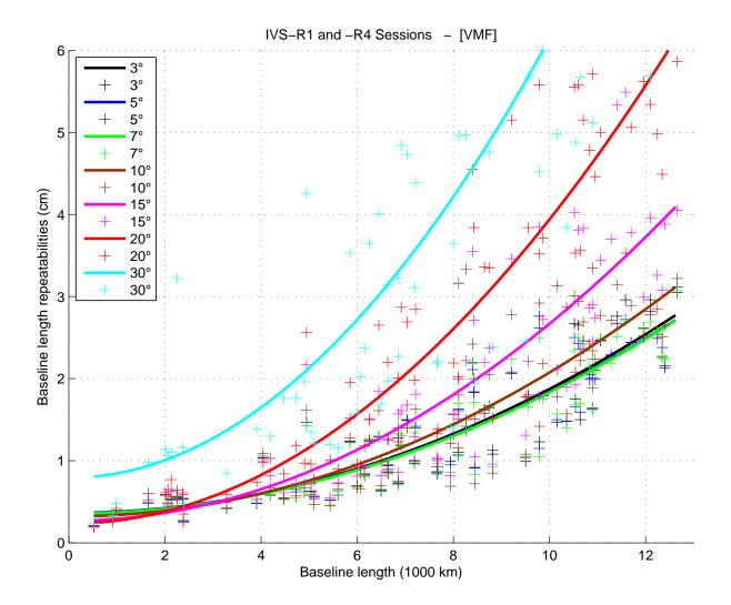
Figure 7.4.: Baseline length repeatabilities with VMF1 for the cut-off angles 3°, 5°, 7°, 10°, 15°, 20°, and 30°.
