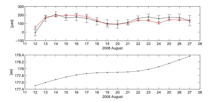
Figure 8.10.: In the upper plot, VieVS daily CPWLO of nutation dX estimates at epochs 0:00 UTC with their formal errors during IVS-CONT08 are shown in red. The daily  $\Delta X_{IERS}$  at epochs 0:00 UTC and their formal errors are shown in black. In the lower plot,  $X_{IAU2000A}$  values at epochs 0:00 UTC are shown. The VieVS analysis options are given in Table 8.2 and 8.3.
