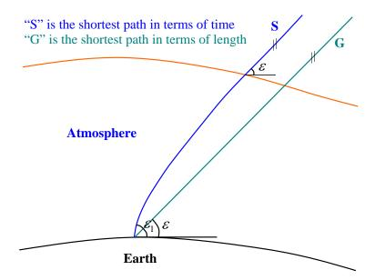
Figure 5.1.: Bending of the ray in the neutral atmosphere. The outgoing (vacuum) elevation angle  $\varepsilon$  is smaller than the initial elevation angle  $\varepsilon_1$  (Böhm, 2004).
