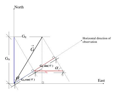
Figure 5.4.: Projecting the gradient vector at the slant direction to the azimuth of observation.
