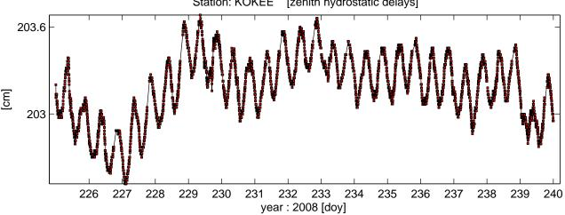
Figure 5.6.: VieVS, ZHD and 30 minutes ZWD estimates of VieVS at Kokee VLBI site - Hawaii, USA during IVS-CONT08. Loose constraints (0.7  $\frac{ps^2}{sec}$  = 11 mm after 30 minutes) are applied.
