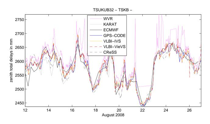
Figure A.6.8.: ZTDs at co-located site Tsukuba in Japan during IVS-CONT08.
