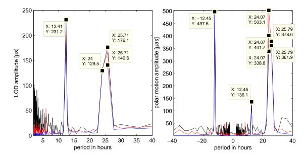
Figure 8.18.: Fourier spectra plots of LOD and polar motion. The blue line shows the spectra of the hourly ERP values from HF-ERP models. The red line shows the spectra of the hourly ERP estimates from GPS. The black line shows the spectra of the hourly ERP estimates from VLBI (VieVS). The LOD were calculated from the time derivatives of  $\Delta UT1$  values of HF-ERP models and dUT1 estimates of VieVS. The VieVS analysis options are given in Tables 8.2 and 8.4.
