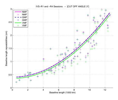
Figure 7.3.: Baseline length repeatabilities with VMF1, GMF, and NMF for a cut-off angle 3°.
