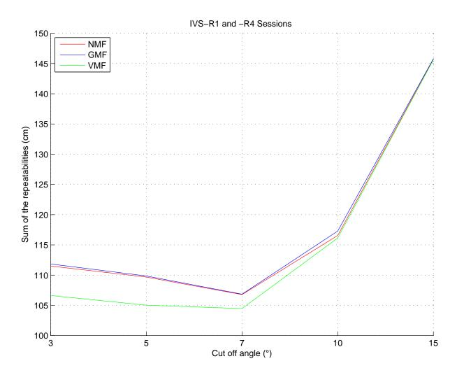
Figure 7.5.: Sum of the baseline length repeatabilities with VMF1, GMF, and NMF for the cut-off angles  $3^{\circ}$ ,  $5^{\circ}$ ,  $7^{\circ}$ ,  $10^{\circ}$ , and  $15^{\circ}$ .
