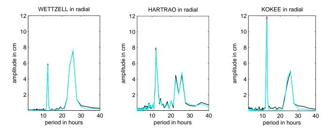
Figure 8.3.: Cyan lines show the Fourier spectra of hourly radial displacements computed from the solid Earth tide model (McCarthy and Petit (2004), Chapter 7.1.1). Black lines show the spectra of the radial components of the hourly CPWLO coordinate estimates when only the solid Earth tide model displacements were not reduced a priori from the observations during IVS-CONT05. The analysis options of the IVS-CONT05 sessions are given in Table 8.1.
