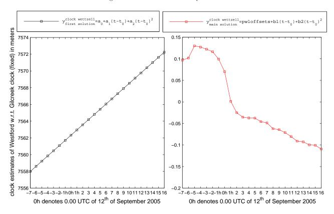
Figure 4.1.: Westford clock errors w.r.t. Gilcreek clock during the first session of IVS-CONT05. The left plot shows the clock polynomial estimated from the first LS solution. The right plot shows the hourly CPWLO estimates plus polynomial with rate and quadratic terms from the main solution. The total clock estimates are the sum of the two plots.
