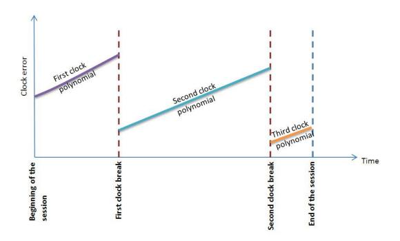
Figure 4.4.: A polynomial is fitted for each interval delimitated by the occurrence time of clock breaks.
