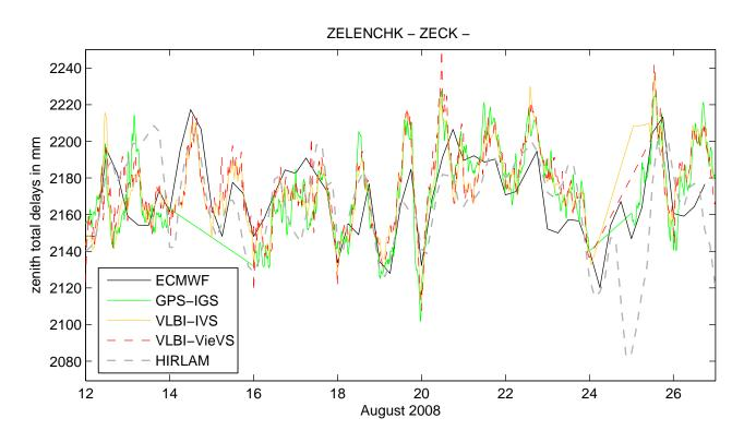
Figure A.6.10.: ZTDs at co-located site Zelenchukskaya in Russia during IVS-CONT08.
