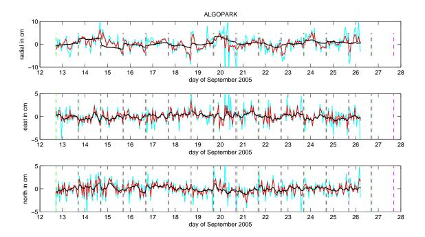
Figure A.8.10.: Black, red and cyan lines show VieVS, hourly (at UTC integer hours) CPWLO coordinate estimates of the VLBI antenna Algopark during IVS-CONT05 when loose constraints were applied on the hourly coordinate estimates as 4 mm/hour, 3 cm/hour, and 21 cm/hour, respectively.
