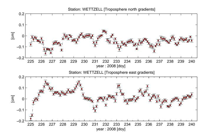
Figure 5.7.: Troposphere north and east gradient estimates of VieVS at Wettzell (Germany), at 6 hour intervals during IVS-CONT08. The a priori north and east gradients are zero. Loose constraints (2 mm/day = 0.5 mm after 6 hours) are applied.
