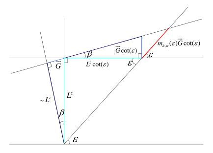
Figure 5.3.: Projecting gradient vector from zenith to slant direction.  $\beta$  is the tilting angle of the mapping function assuming a horizontally stratified atmosphere (Böhm, 2009).
