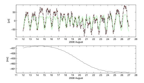
Figure 8.15.: In the upper figure, grey bars show the VieVS hourly (at UTC integer hours) CPWLO dUT1 estimates with their formal errors during IVS-CONT08. The total hourly  $\Delta UT1$  values of the HF-ERP models are shown in the same plot in green. In the lower plot, linearly interpolated  $\Delta UT1_{IERS}$  plus VieVS hourly CPWLO dUT1 estimates are shown. The VieVS analysis options are given in Tables 8.2 and 8.4.
