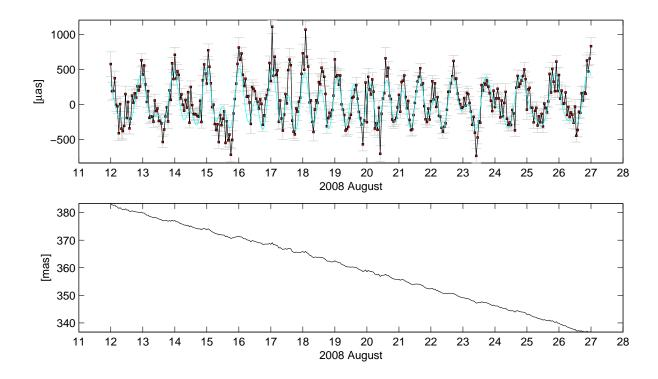
Figure 8.14.: In the upper figure, grey bars show the VieVS hourly (at UTC integer hours) CPWLO  $dy_p$  estimates with their formal errors during IVS-CONT08. The total hourly  $\Delta y$  values of the HF-ERP models are shown in the same plot in cyan. In the lower plot, linearly interpolated  $(y_p)_{IERS}$  plus VieVS hourly CPWLO  $dy_p$  estimates are shown. The VieVS analysis options are given in Tables 8.2 and 8.4.
