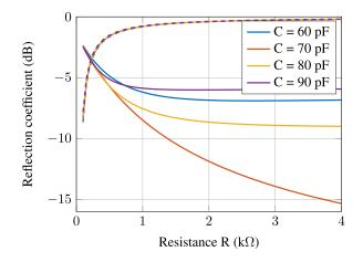
FIGURE 7. Comparing reflection coefficients of different loads with (solid) and without (dashed) a two port network at 13.56 MHz.
