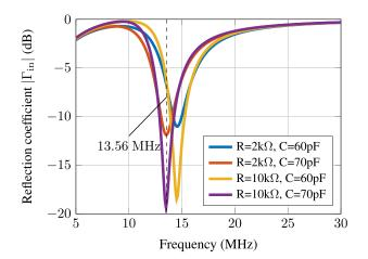
FIGURE 6. Comparing the reflection coefficients of different loads connected to a two port network.
