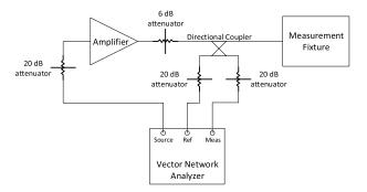
FIGURE 8. Test setup for characterizing the IC.
