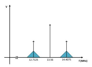
FIGURE 12. Frequency spectrum during load modulation.
