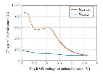
FIGURE 16. The measured unloaded and loaded resistances of the IC.
