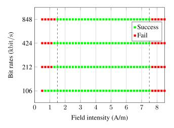
FIGURE 22. Results of standardized test on the optimized card.
