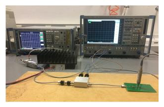
FIGURE 10. Implemented test setup for the de-embedding transformer-based method.
