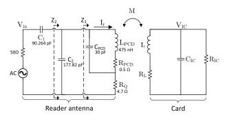
FIGURE 17. Circuits of the reader and card.
