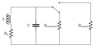
FIGURE 3. Simplified circuit model of an HF RFID card with IC.
