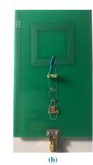
FIGURE 9. Manufactured PCB for characterizing the IC using de-embedding transformer-based method (a) Top (b) Bottom.
