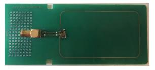
FIGURE 19. A calibration coil with an IC.
