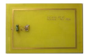
FIGURE 1. Manufactured "Card 1" with a 69 pF IC.
