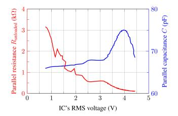
FIGURE 11. Equivalent load of the IC.
