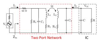
**FIGURE 5.** Circuit model of the de-embedding transformer-based measurement fixture.
