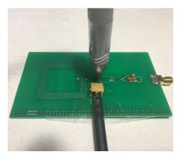
FIGURE 14. Manufactured PCB with current and voltage probes.
