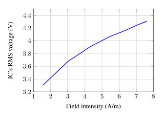
FIGURE 23. Simulated IC's voltage of optimized RFID card at 27 dBm reader's power and varying the coupling factor from 5% to 50%.
