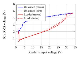
FIGURE 18. Comparison between measurements and simulations of the IC's voltage.
