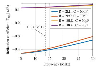
FIGURE 4. Reflection coefficients for 4 variants of an RC shunt circuit.
