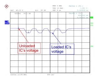
FIGURE 15. Measuring IC's voltage during load modulation using signal analyzer.
