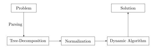
Figure 3. Dynamic-programming approach based on tree-decompositions.
