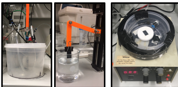
humidity was adjusted using a gas flow adjuster with a dry air and a wet air flow. Humidity was checked in the box before spinning. For spin coating the beforehand cut silicon wafers were inserted onto the home printed sample holder, the lid was closed, spinning with constant speed (e.g. 2000 rpm) was started. Subsequently, 50 \mu\text{L} of the sol solution were deposited on top of the rotating substrate. After 30 seconds rotating in the Figure 43: left/middle picture: home-built Dip-Coater, “Dippert 3000” right picture: Spin coater equipped with a plastic box
