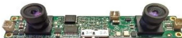
Figure 57: Stereo-cameras used for the robot realization. (Leopard Imaging, last retrieved 2015)
