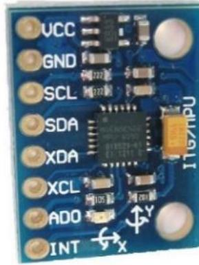
Figure 58: The MPU 6050 IMU (MPU 6050, last retrieved 2018)
