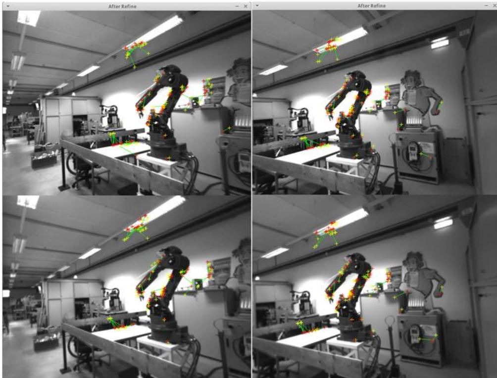
Figure 78: PTAM result with the stereo-cameras in bad lightning condition
