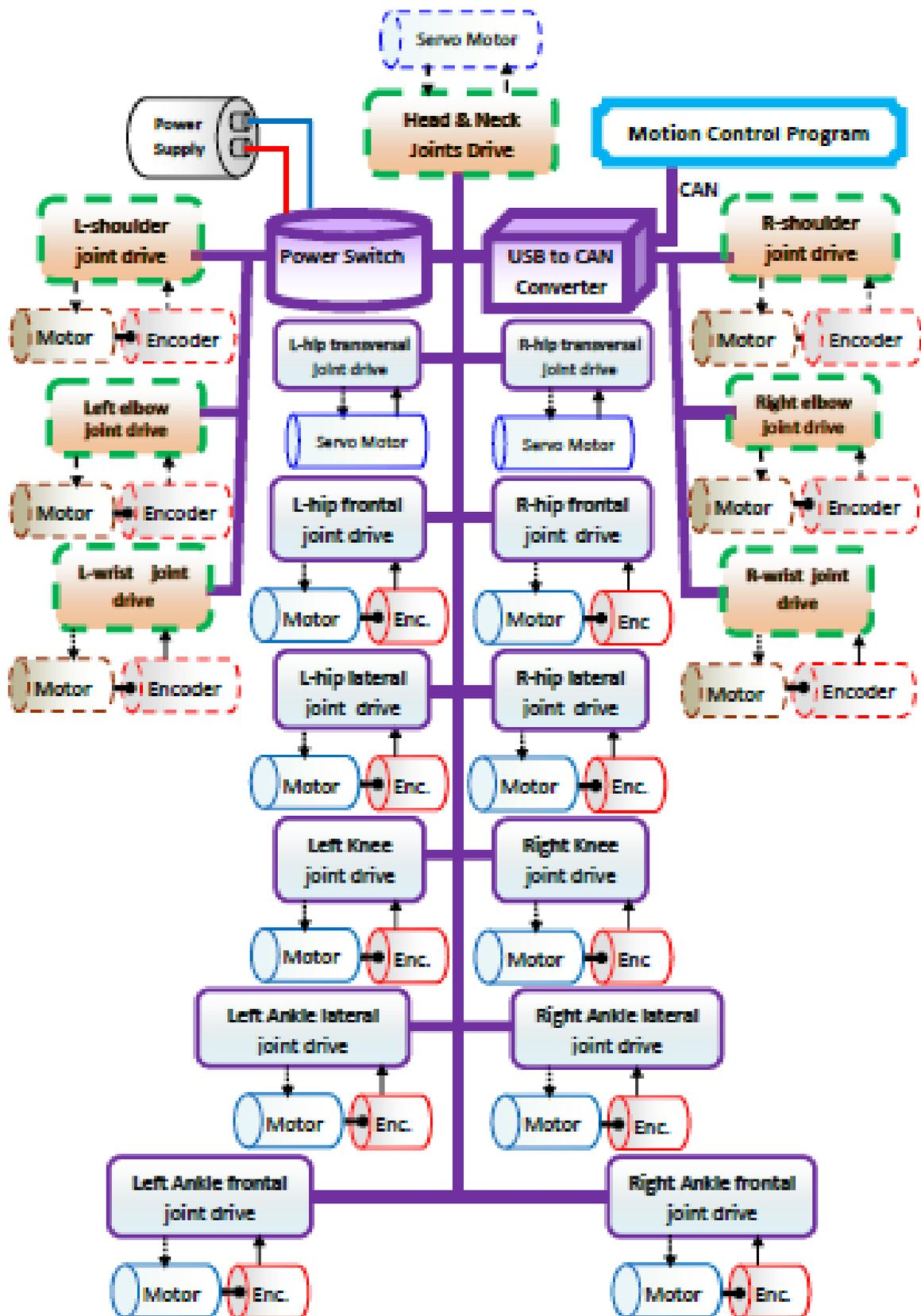
Figure 19: Scheme of Archie hardware (Dezfooli, 2013)
