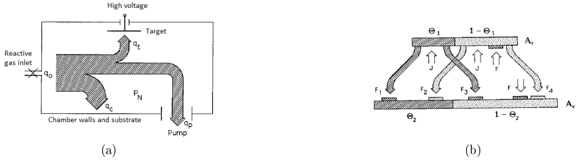
Figure 63: schematic illustration of the Berg-model; (a) contributions to the total reactive gas flow q_0 , where q_t is the fraction poisoning the target, q_c the chamber and q_p the fraction pumped out without interaction, in total the chamber pressure rises to p_R for a general gas and p_N for nitrogen as primarily used by Berg; (b): fractional poisoned areas \theta_1 , \theta_2 and mettalic areas 1 - \theta_1 , 1 - \theta_2 of the target with total area A_t and chamber with total area A_c respectively, J describes the argon atoms sputtering from the target and F the adsorbed oxygen ions at the target and the chamber; F_i denote the particle flows from the target to the surface fractions; adapted from [20, 19]
