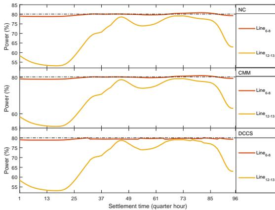
(a) High loaded lines flow for load profile 1
