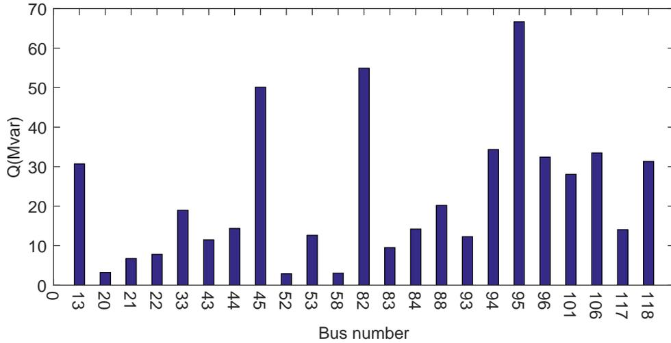
Figure 5.19: Reactive power injection of FACTS in IEEE 118 bus system
