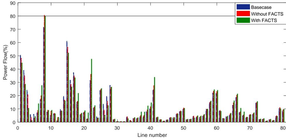
Figure 5.13: Power Flow on lines in IEEE 57 bus system
