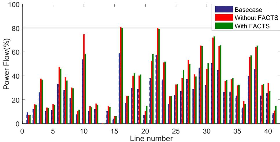
Figure 5.2: Power Flow on lines in IEEE 30 bus system
