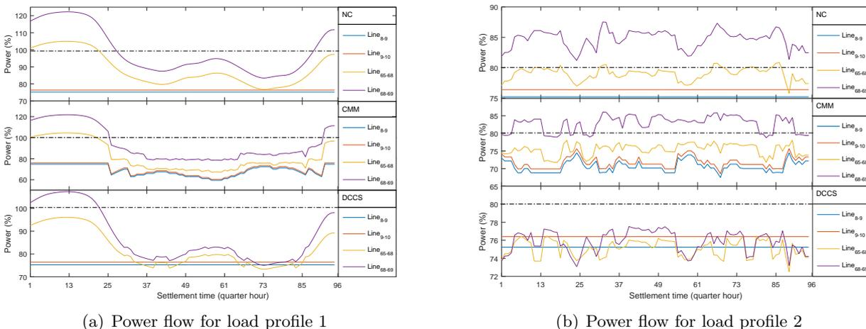
Figure 6.15: Dynamic power flow over high loaded lines of IEEE 118 bus system in load profiles
