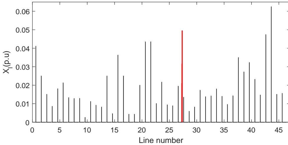
Figure 5.10: Reactance of lines in IEEE 39 bus system
