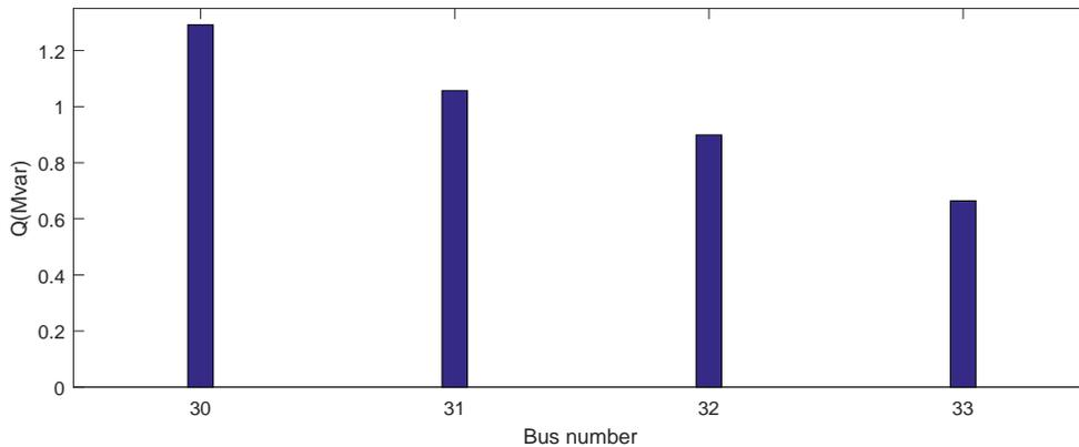
Figure 5.15: Reactive power injection of FACTS in IEEE 57 bus system
