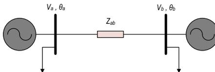
**Figure 2.1:** Transmission line connecting two areas
