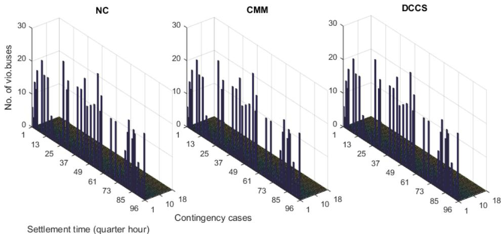
Figure 6.22: Over voltage buses of IEEE 300 bus system in contingency cases for Load profile 2
