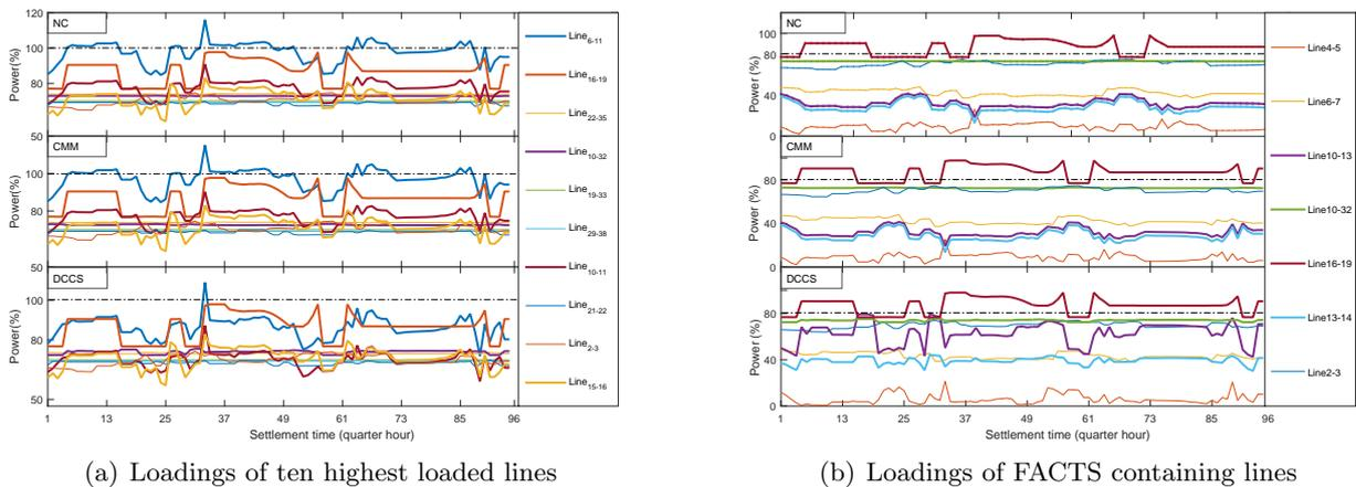
Figure 6.8: Dynamic power flow of IEEE 39 bus system for load profile 2
