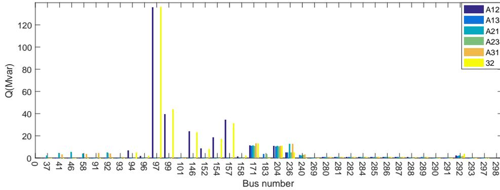
Figure 5.30: Reactive power injection of FACTS in IEEE 300 bus system
