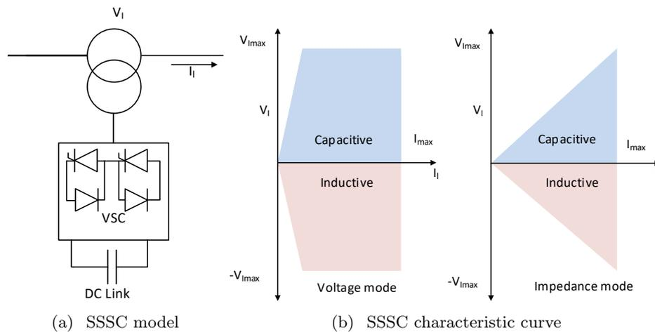
Figure 2.6: Static Synchronous Series Compensator SSSC
