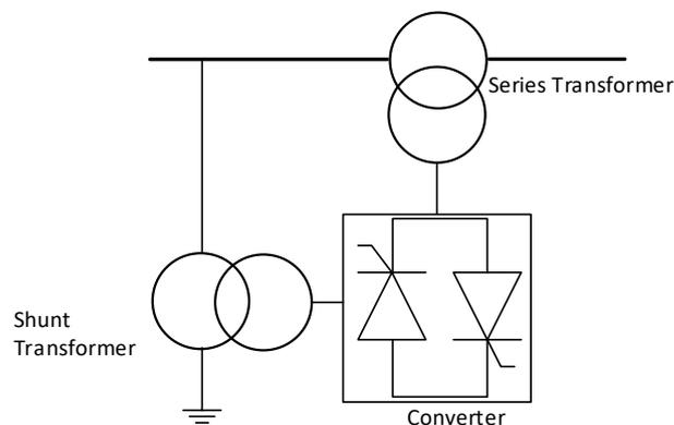
Figure 2.7: Thyristor Controlled Shifting Transformer TCPST
