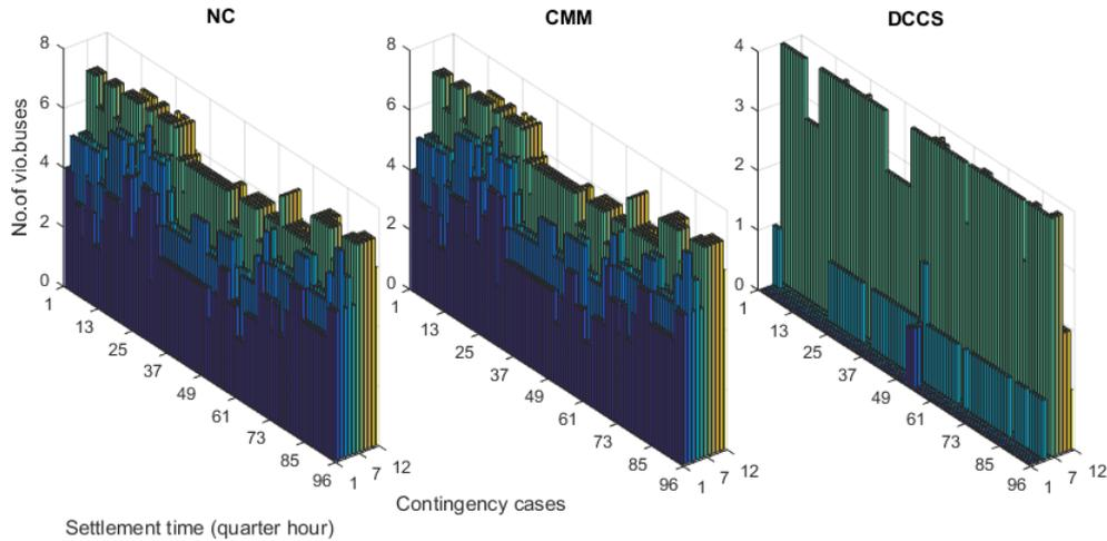
Figure 6.18: Violated buses of IEEE 118 bus system in contingency cases for Load profile 2
