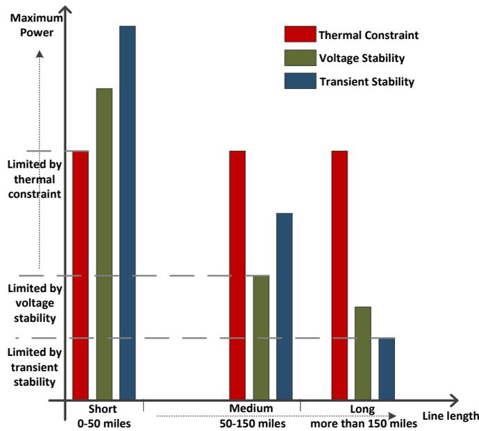
Figure 1.2: Constraints for Transmission Capability
