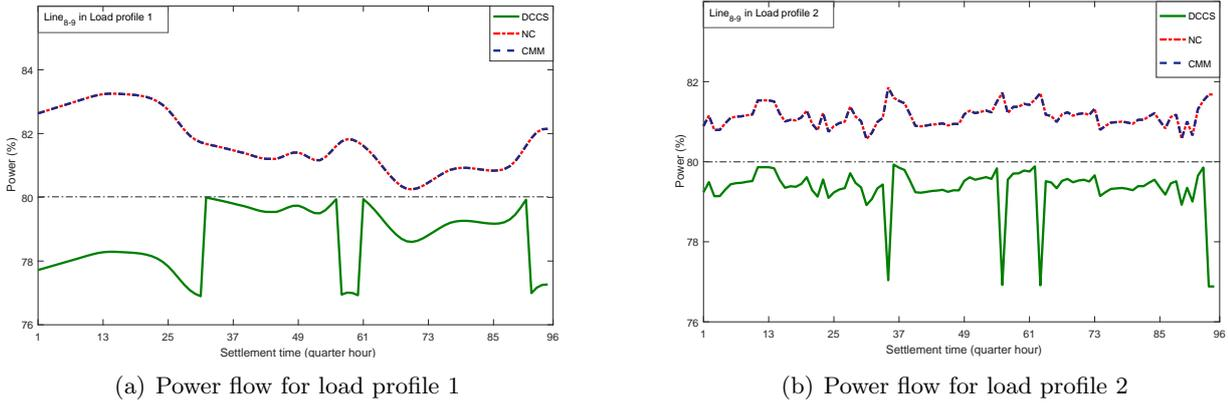
Figure 6.11: High loaded lines of IEEE 57 bus system in both load profiles
