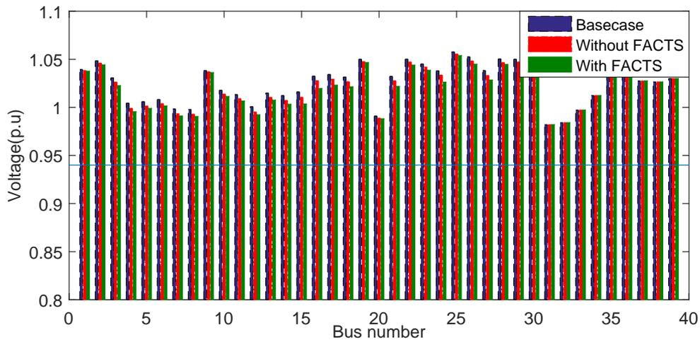
Figure 5.11: Voltage magnitude of buses in IEEE 39 bus system
