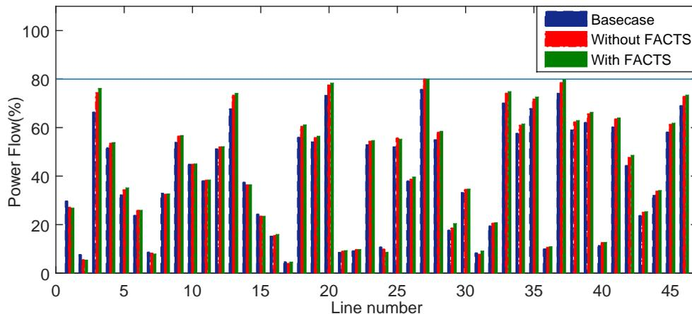
Figure 5.9: Power Flow on lines in IEEE 39 bus system
