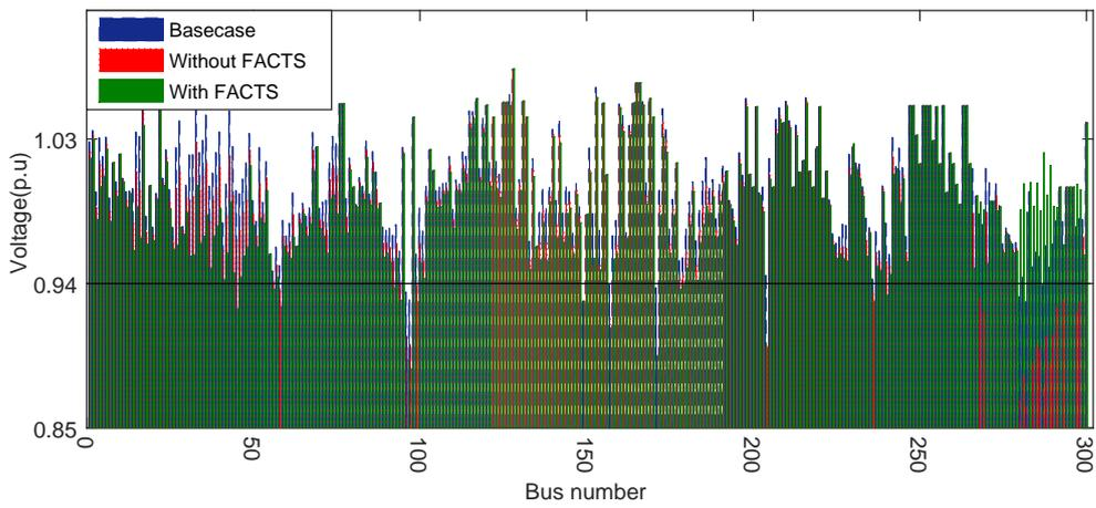
Figure 5.23: Voltage magnitude of buses in IEEE 300 bus system
