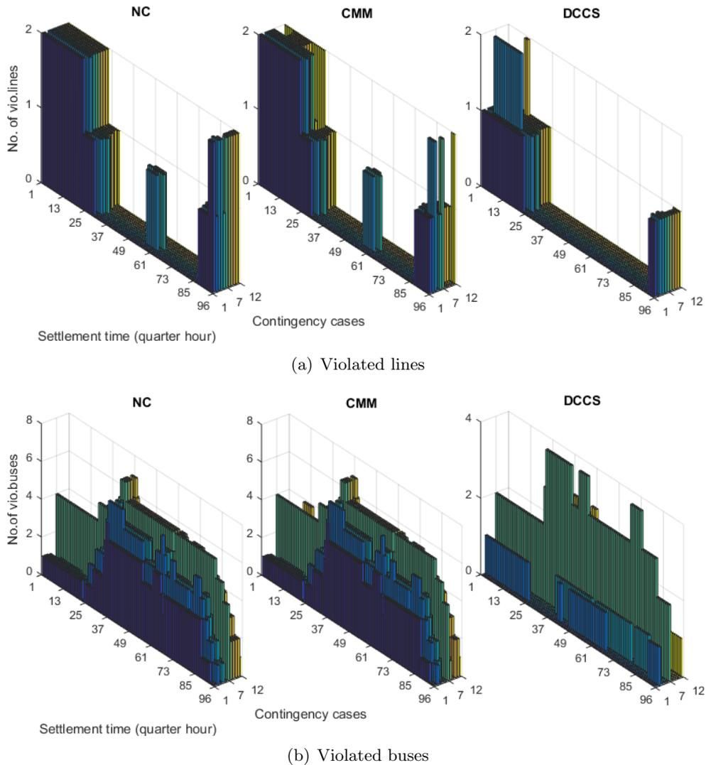
Figure 6.17: Violated lines & buses of IEEE 118 bus system in contingency cases for Load profile 1
