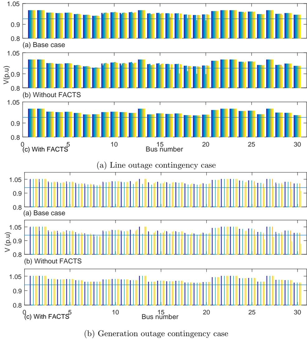
**Figure 5.7:** Bus voltages of contingency cases in IEEE 30 bus system
