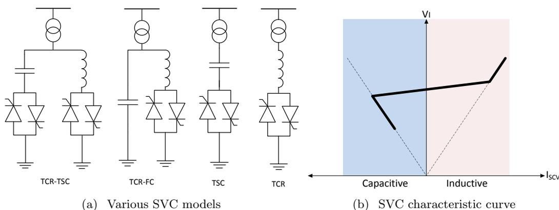
**Figure 2.3:** Static Var Compensator SVC
