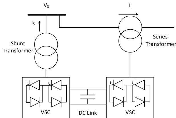
**Figure 2.8:** Unified Power Flow Controller UPFC models
