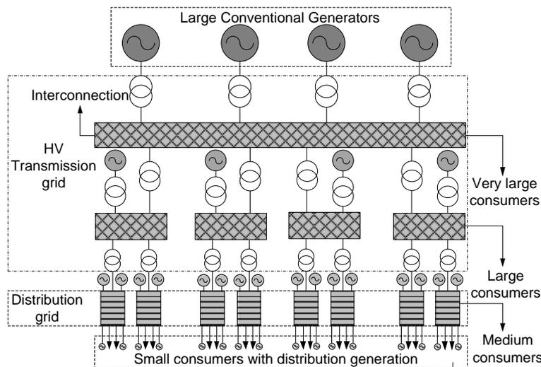
Figure 1.1: Conventional power system structure with expected distributed generation
