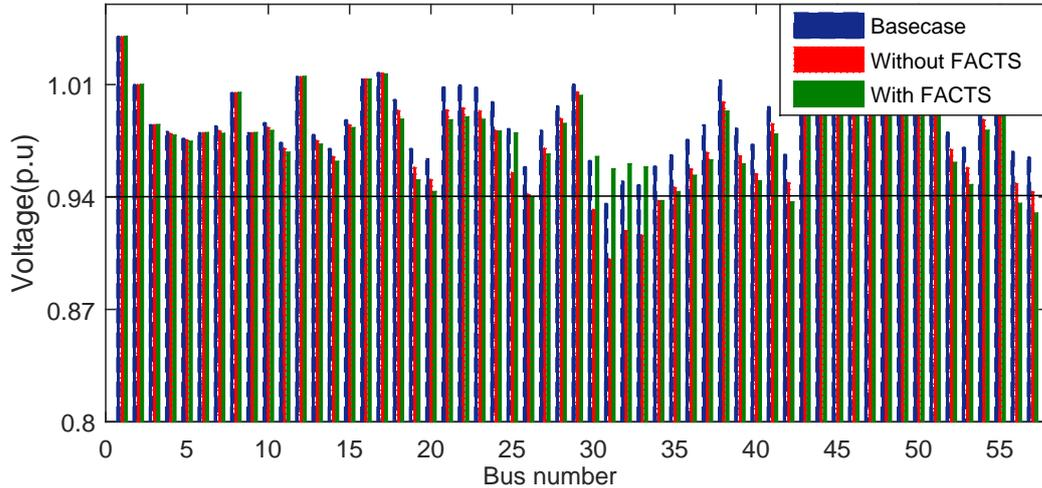
Figure 5.14: Voltage magnitude of buses in IEEE 57 bus system
