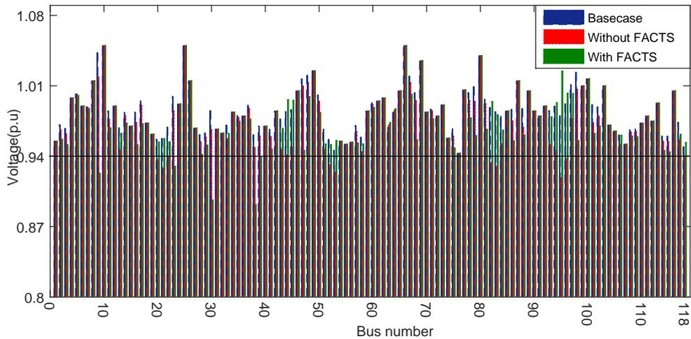
**Figure 5.18:** Voltage magnitude of buses in IEEE 118 bus system
