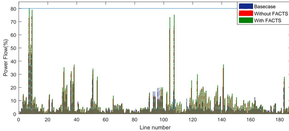
**Figure 5.17:** Power Flow on lines in IEEE 118 bus system
