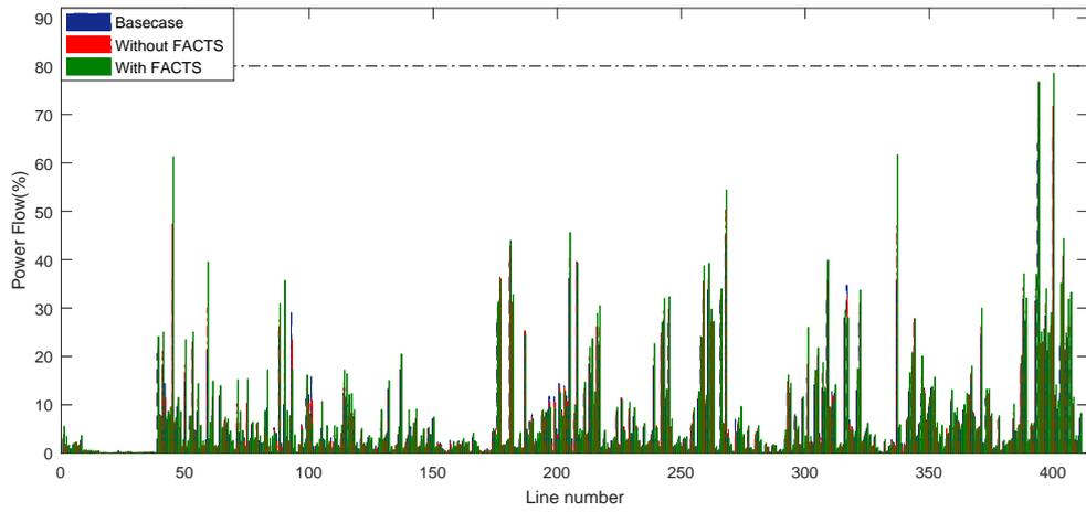
Figure 5.21: Power Flow on lines in IEEE 300 bus system
