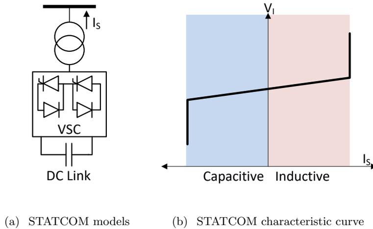
**Figure 2.4:** Static Synchronous Compensator STATCOM
