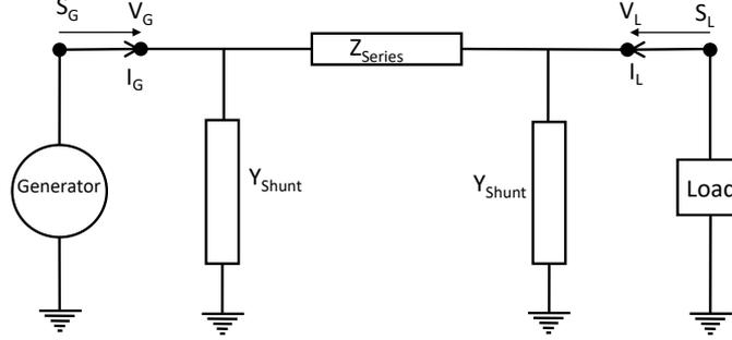
Figure 3.1: Transmission line model
