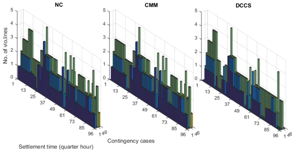
**Figure 6.9:** Lines violation of IEEE 39 bus system in line outages contingency cases for load profile 2
