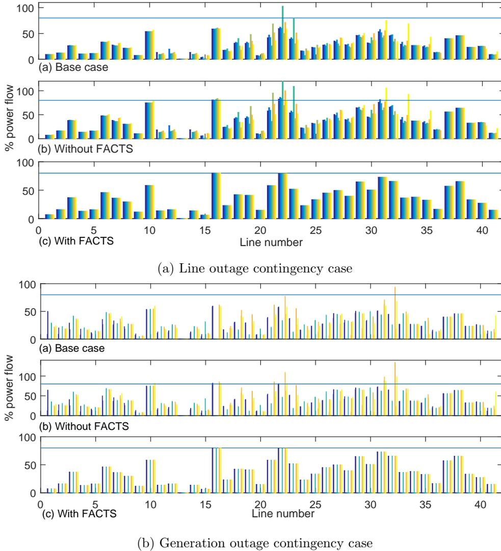
**Figure 5.3:** Power flow of contingency cases in IEEE 30 bus system
