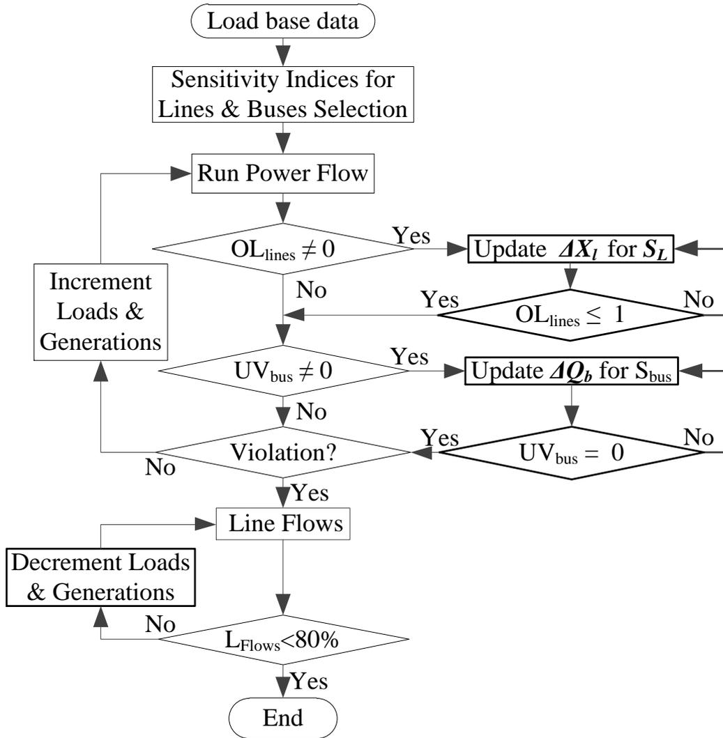
Figure 3.3: Flowchart of Modified RFP for *TTC* Enhancement
