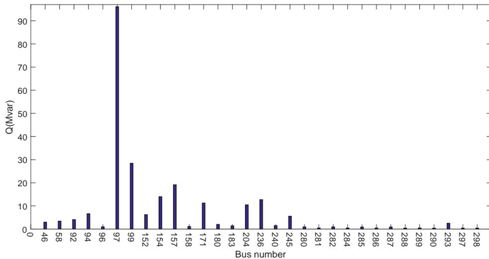
**Figure 5.25:** Reactive power injection of FACTS in IEEE 300 bus system
