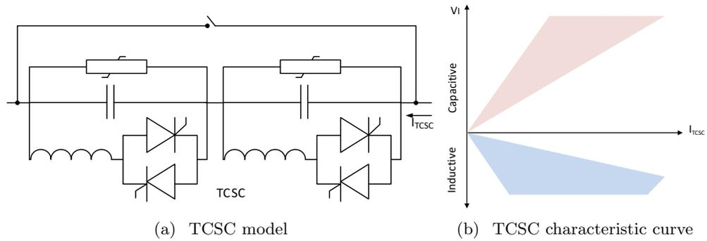
Figure 2.5: Thyristor Controlled Series Compensator TCSC
