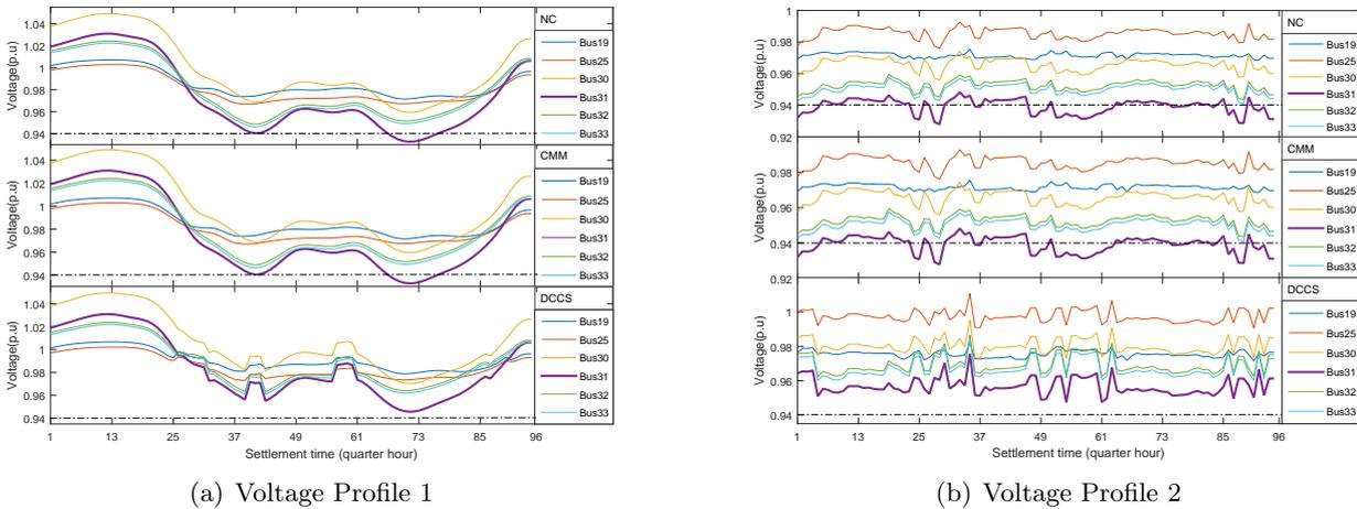
Figure 6.12: Dynamic Voltage profiles of IEEE 57 bus system for both load profiles
