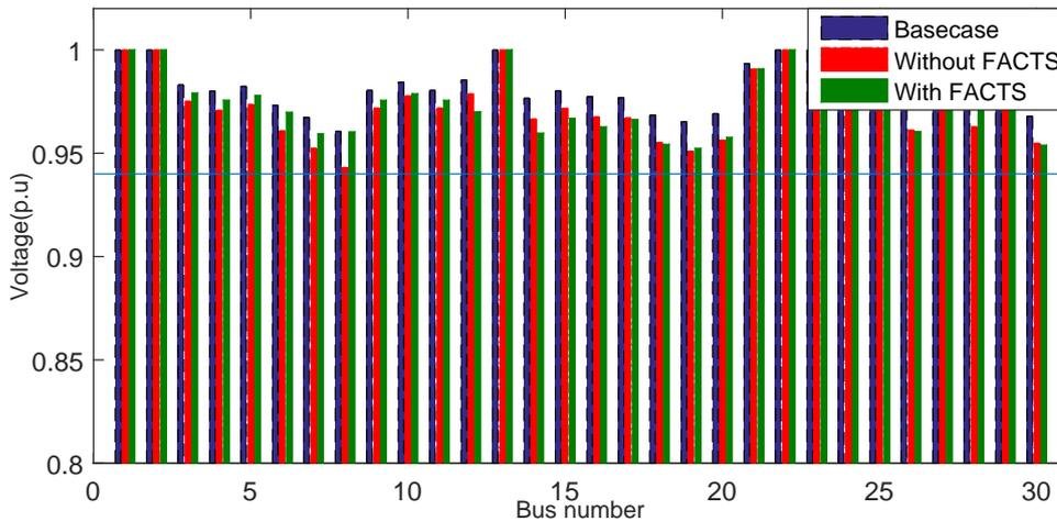
Figure 5.5: Voltage magnitude of buses in IEEE 30 bus system
