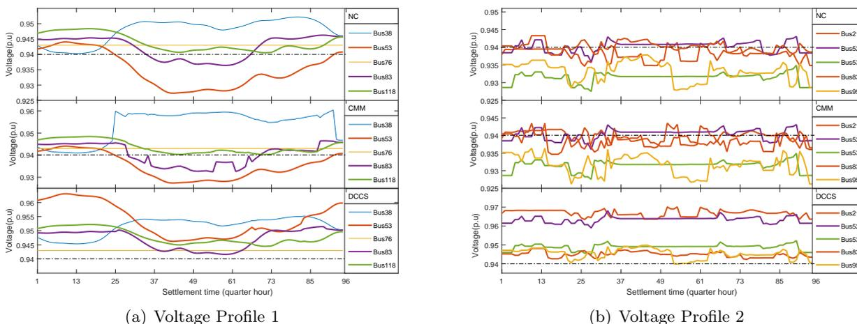
Figure 6.16: Dynamic Voltage profiles at violating buses of IEEE 118 bus system
