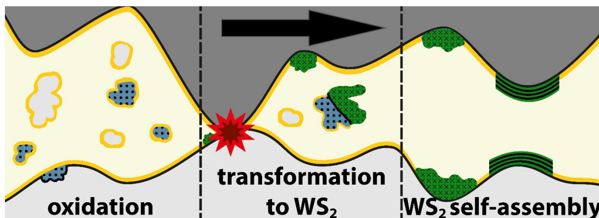
Figure 40: Highlight I, reaction pathway for the in-situ generation of \text{WS}_2
