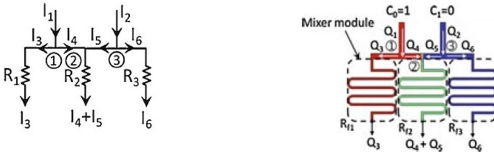
Figure 10: Similarity between electric circuit and hydraulic circuit [14].
