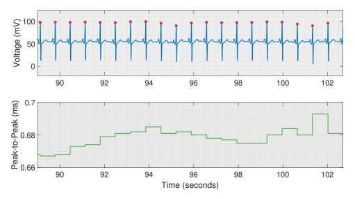
Fig. 2.3.8.: The graph shows an artefact free ECG, as one would see it using the MAT-LAB code for signal processing: the red dots are generated by the automatic R-peak detection. The green graph shows the corresponding time between two R-peaks, also known as *interbeat interval*. All HRV parameters are calculated from this peak-to-peak time.
