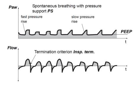
Fig. 3.4.2.: Variable PS works on the same basis as SPN-CPAP/PS but differs the with every breath applied pressure support within a preset range, without exceeding the maximum pressure or falling below the PEEP level. Image taken from [47].
