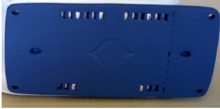
FIGURE 4.22: Squashed module after lamination and sintering when using the required lamination pressure for layer adhesion.
