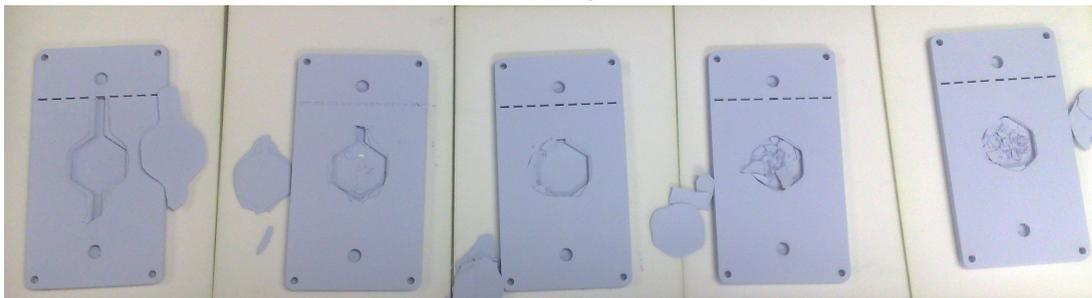
FIGURE 4.25: Heater module incorporating sacrificial material after binder burnout
