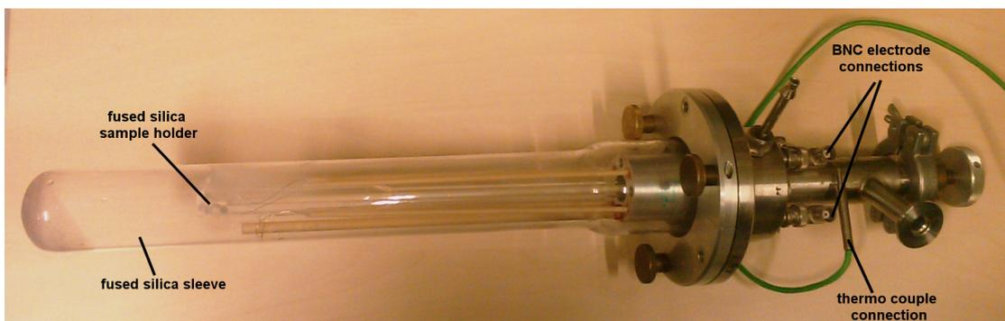
FIGURE A.11: Measurement assembly.
