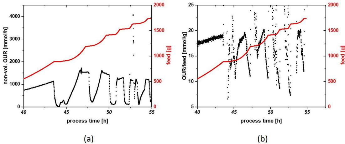
Figure 21: (a) Non volumetric OUR as a function of linear increasing  $q_{s,c}$  values during induction phase (exponential increase in mass feed – red). Sugar accumulation in the broth leads to flattening of the OUR signal; (b) OUR normalized to fed mass of glycerol. A drop in the signal indicates sugar accumulation and can be used as trigger for the dSn based control. Sugar digestion capacity is constantly decreasing over time.
