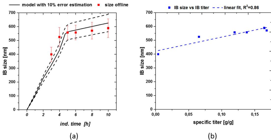
Figure 27: (a) Size modeling including real measured data with standard deviations. Especially early sizes could only be described using the model-based approach; (b) Size-titer correlation for fermentation with feeding strategy implied in Figure 3 a.
