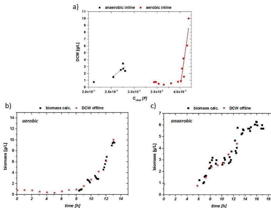
**Figure 7.** (a) Impedance signal vs. offline DCW for aerobic (circles) and anaerobic (squares) cultivations with linear fits beyond a threshold of 1 g/L DCW. (b) Impedance signal of aerobic run (smoothed), calculated via a linear fit into a viable biomass. This is correlated to the offline DCW. (c) Impedance signal vs. DCW of the anaerobic run.
