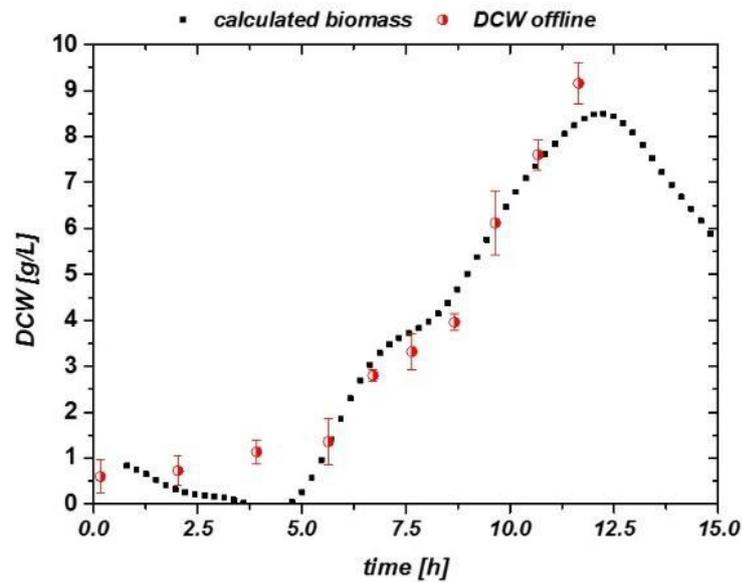
Figure 38: impedance signal vs. DCW of the inline probe in complex media malt extract. A good description is found beyond 1 g/L DCW in this experiment.
