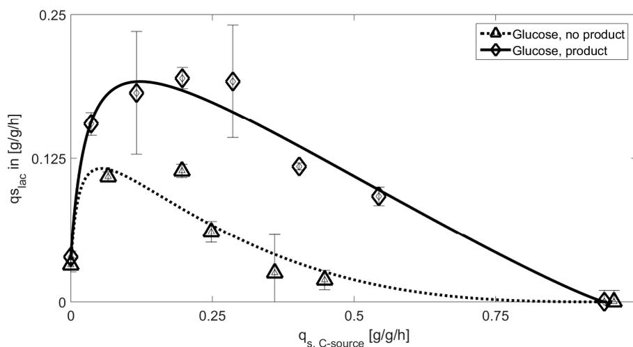
**Figure 3.** Extracted datapoints for  $q_{s,C}$  values including standard deviations for cultivations with glucose using the product producing (glucose product) and the NP strain (glucose, no product). Solid lines represent the model based approach for inducer uptake rates vs. feeding rates models of glucose. A clearly visible difference can be observed during these cultivations.
