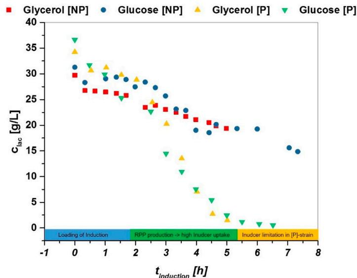
**Figure 2.** High-pressure liquid chromatography (HPLC)-based data for decrease of lactose in fermentation broth exhibiting very similar  $q_{s,C}$  values in [g/L]. A significant decrease over the time of induction is visible in producing (P) strains, while the decrease is way slower in non-producing (NP)-strain-cultivations.
