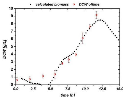
**Figure 9.** Impedance signal vs. DCW for the inline probe in complex medium: malt extract. A good description is found beyond 1 g/L DCW in this experiment.
