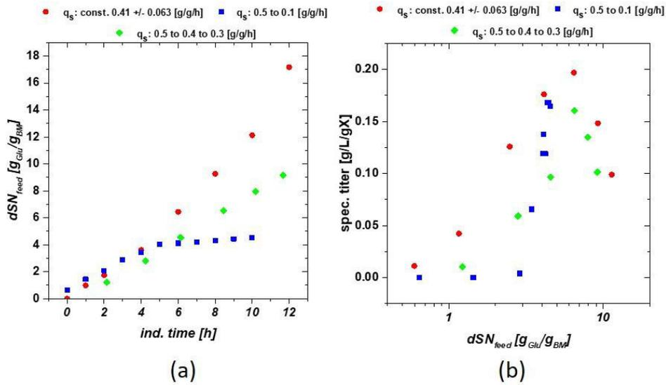
Figure 20: (a) Feeding strategy of three representative cultivations. The change in exponential feeding was triggered at a  $dSn$  of 3.5 g/g; (b) Specific titer for constant  $q_{s,c}$ , instant drop and stepwise drop. Highest titers could be found at instant drop strategy.
