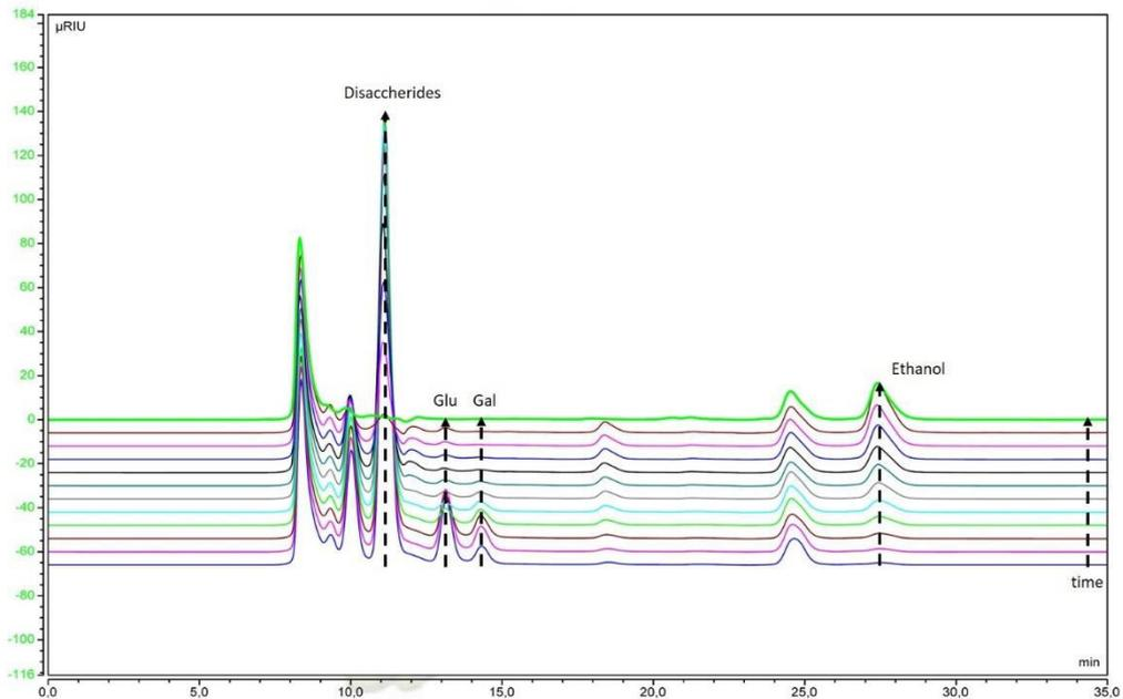
Supplementary 5: HPLC data for malt extract analysis used in sensor development.
