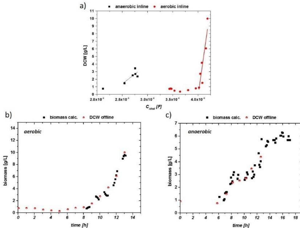
Figure 36: a) Impedance signal vs. offline DCW for aerobic (circles) and anaerobic (squares) cultivation with linear fits beyond a threshold of 1 g/l DCW; b) Impedance signal of aerobic run (smoothed) and calculated via linear fit into a viable biomass. This is correlated to the offline DCW; c) impedance signal vs. DCW of the anaerobic run
