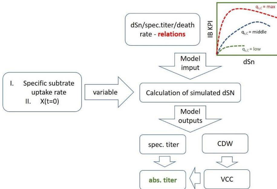
Figure 22: Empirical relations derived from static  $q_{s,c}$  experiments. Induction phase variables are the applied  $q_{s,c}$  during for the cultivation and the biomass before induction phase. Calculation of absolute titers are performed using the VCC approximation during induction.
