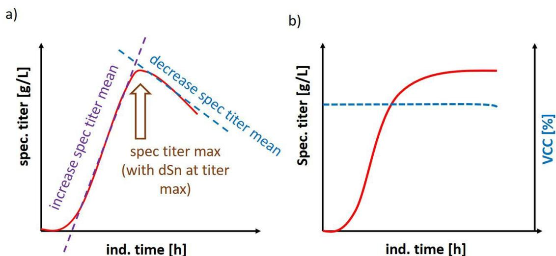
Figure 28: a) sketch of the important time dependent parameters of the KPI spec. titer. All other values are maxima (like size) or at induction time of 12 hours; b) Desired fed-batch behavior, with no visible degradation of spec. titer and high VCC concentration during the whole induction time.
