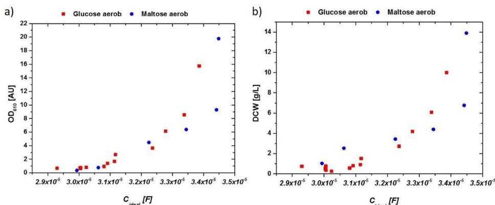
**Figure 3.** (a) OD<sub>610</sub> vs. extracted capacitance of the impedance signal in aerobic cultivations with glucose and maltose. (b) DCW vs. extracted capacitance of the impedance signal in aerobic cultivations. Very similar responses are obtained for both cultivations, irrespective of the used C-source.
