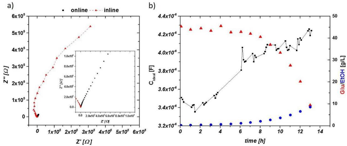
Figure 35: a) Impedance raw-data in Nyquist plot for an aerobic cultivation. Black squares represent signal from the online probe – enlarged in the inlay –, red triangles the inline probe at similar time stages. Capacitance of the inline probe is one order of magnitude lower (as a result of smaller electrode areas.); b) the dependence of impedance signal (not smoothed), glucose consumption and ethanol production in an aerobic cultivation using the inline probe.
