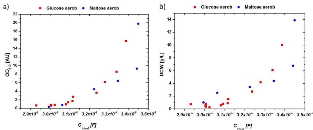
Figure 32: a)  $OD_{610}$  vs. extracted capacitance of impedance signal in aerobic cultivations with glucose and maltose.; b) DCW vs. extracted capacitance of impedance signal in aerobic cultivation. Very similar responses are obtained for both cultivations irrespective of the used C-source.
