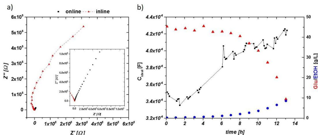
**Figure 6.** (a) Impedance raw data in the Nyquist plot for an aerobic cultivation. Black squares represent the signal from the online probe—enlarged in the inlay—and red triangles, the inline probe at similar time stages. Capacitance of the inline probe is one order of magnitude lower (as a result of smaller electrode areas). (b) The dependence of the impedance signal (not smoothed), glucose consumption and ethanol production in an aerobic cultivation using the inline probe.
