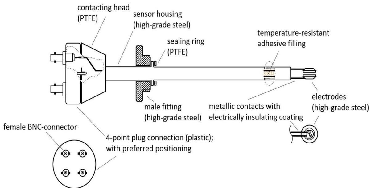
Figure 30: Sketch of the inline probe prototype indicating used materials and wiring. Connection to the impedance analyzer was performed using 4-point BNC “Bayonet Neill Concelman” connection.
