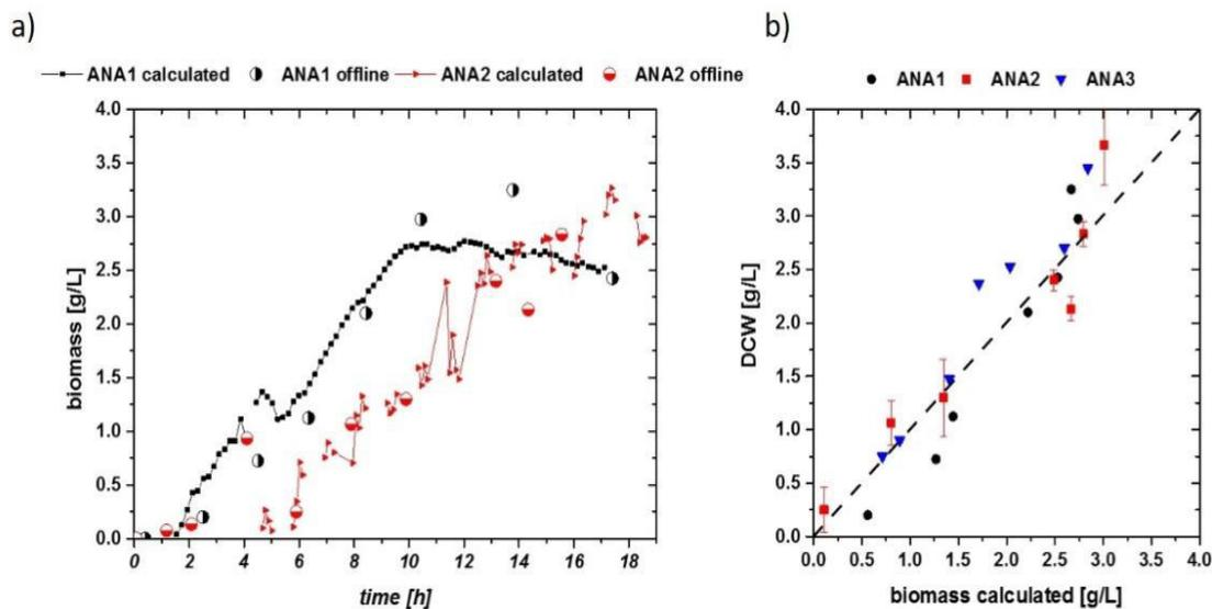
Figure 34: a) biomass calculated of the impedance signal fit extracted in Fig. 4 a) including offline measured DCW values as circles. Flow cytometric measurements confirmed that no dead population is visible, so DCW can be compared to the viable cell concentration in these runs; b) residual analysis of the three anaerobic runs. Despite the low cell densities, a very accurate correlation can be found in all cultivations. Error bars are exemplarily plotted for ANA2 cultivation.
