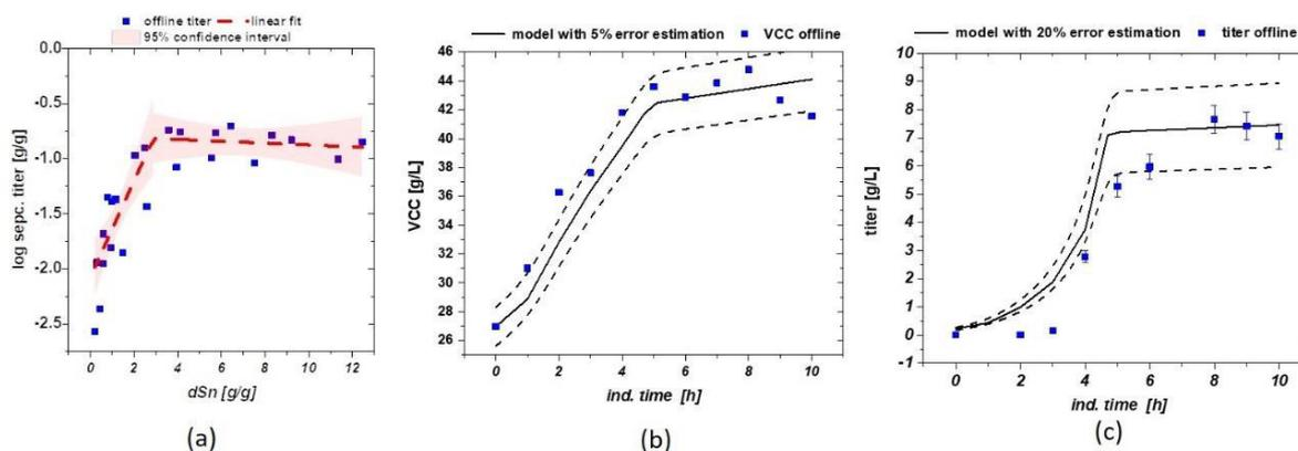
Figure 23: (a) Data driven model for specific titer of the N-Pro fused model protein, including 95% confidence interval. A bilinear fit is used for description of the log(specific titer); (b) VCC model with 5% error estimation including data from FCM measurement, (c) titer calculated via VCC. Late model values fit well to offline measured titers.
