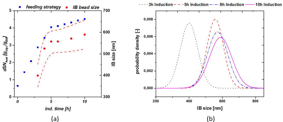
Figure 26: (a) Model cultivation with change in the  $q_{s,c}$  from 0.5 g/g/h to 0.1 g/g/h at a dSn value of about 4 g/g. The lower  $q_{s,c}$  value results in a high viable cell concentration at late induction times; (b) probability density plot of cultivations as a function of induction time
