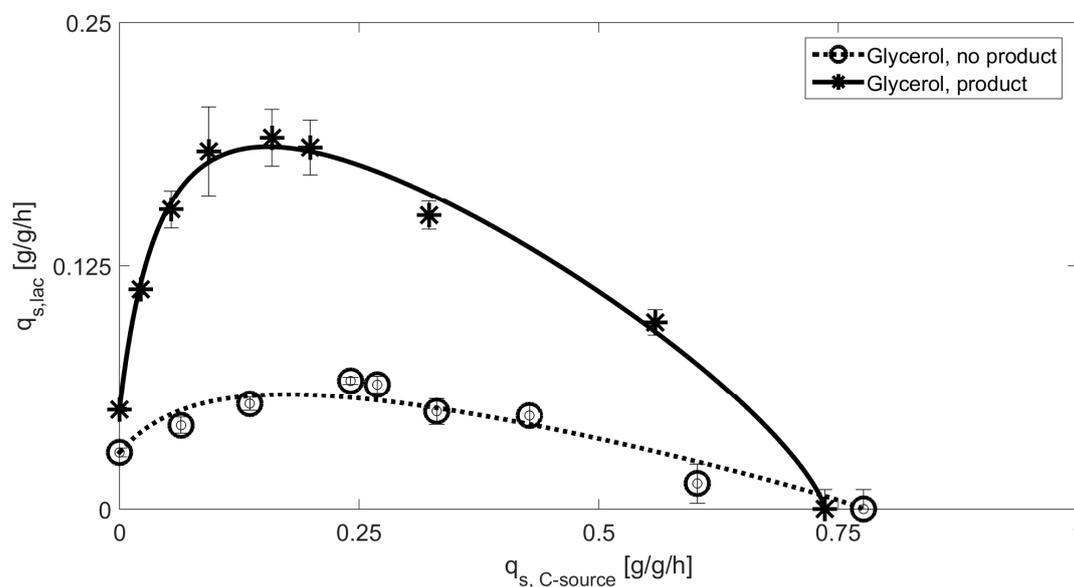
**Figure 4.** Extracted datapoints for  $q_{s,C}$  values including standard deviations for cultivations with glycerol using the product producing (glycerol, product) and the NP strain (glycerol, no product). Solid lines represent the model based approach for inducer uptake rates vs. feeding rates models of glucose.
