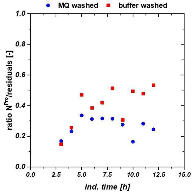
Supplementary 1: Analysis of the first center point run representing IB purity. Buffer washed samples showed generally higher purity. Differences in size and titer are within the given standard deviation.
