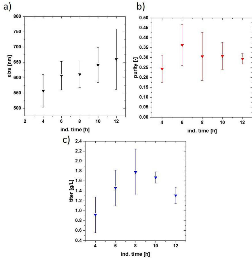
Supplementary 3: a) Mean value for size and deviations of the three individual center point runs. Error stays constant; b) purity-based analysis, with decreasing error over time; c) titer-based analysis. Error decreases drastically in later time stages (range of constant titer or even proteolytic degradation).
