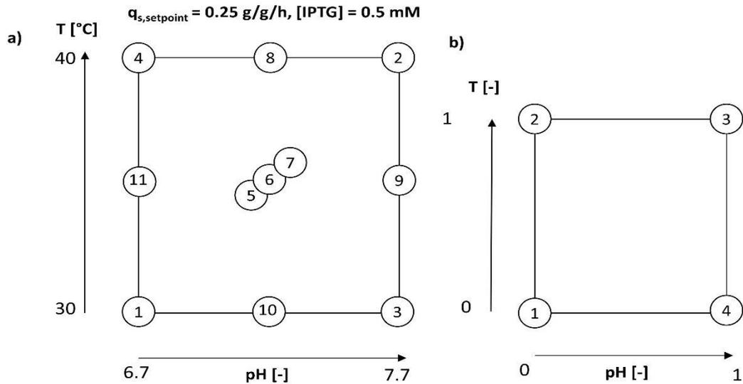
Figure 4: DoE for determination of the influence of classical process parameters on IB QAs. Starpoints (8,9,10,11) were performed in a DasGip parallel system, while the others were cultivated in a stainless-steel Sartorius Stedim reactor; b) reduced design space for *strain 2* based on optimal cultivation parameters.
