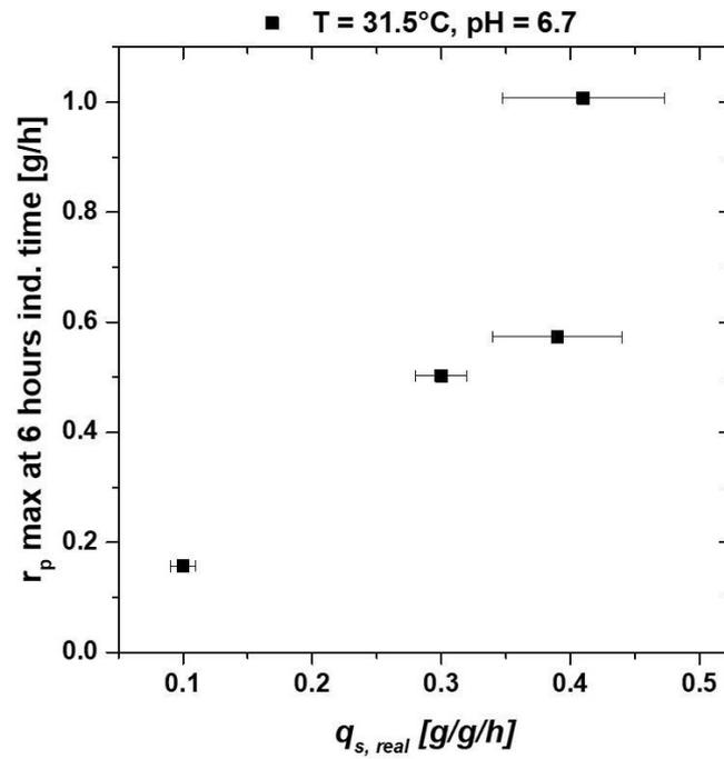
Supplementary 4:  $q_{s,real}$  with standard deviation based on the reverse analysis. The higher the  $q_s$  the higher is the error, due to onset of degradation and sugar accumulation in the broth. A rising trend can be deduced from these measurements.
