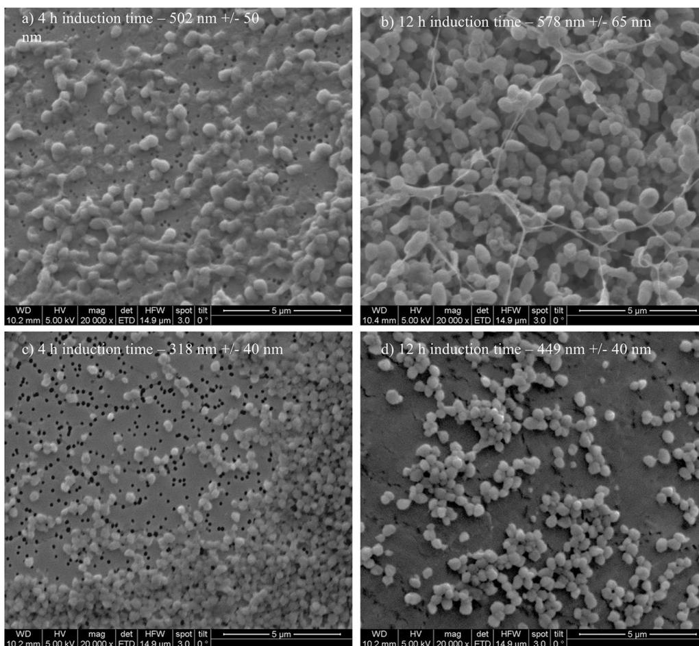
**Fig. 2** Extracted IBs filtered onto Au coated polycarbonate filter and analyzed using SEM for 4 h induction time and 12 h induction time. Strong difference in size can be spotted for the two-time points
