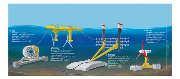
**Figure 33:** Tidal Power plant Systems (from https://www.canadiangeographic.ca/ article/nova-scotias-first-stream-tidal-turbine-starts-producing-power)
