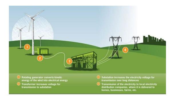
Figure 8: How wind turbines work (from https://canwea.ca/wind-facts/why-wind-works/)
