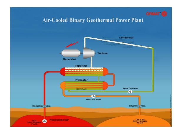
**Figure 28:** Air Cooled Geothermal Power Plant (from http://geo-energy.org/basics.aspx)
