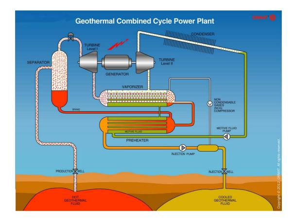
**Figure 29:** Geothermal Combined Cycle Power Plant (from http://geo-energy.org/ basics.aspx)
