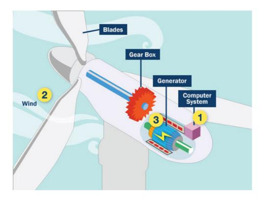
Figure 9: Components of a wind Turbine (from http://www.industrycrane.com/ blog/.html)
