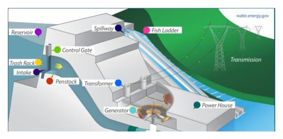
**Figure 30:** Hydroplant System Diagram (from http://gubik.abidingtruthministry.co/ hydropower-works/)
