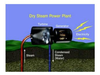
Figure 27: Dry Steam Power Plant Sys (from http://geo-energy.org/basics.aspx)
