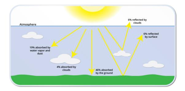
**Figure 12:** Solar Energy (from http://www.smartenergytoday.net/industryknowledge/ solar-energy/solar-energy-absorbtion-2/)
