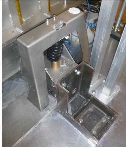
Figure 7.3.: Additional L-shaped fixing of the vacuum chamber to the UCN platform.
