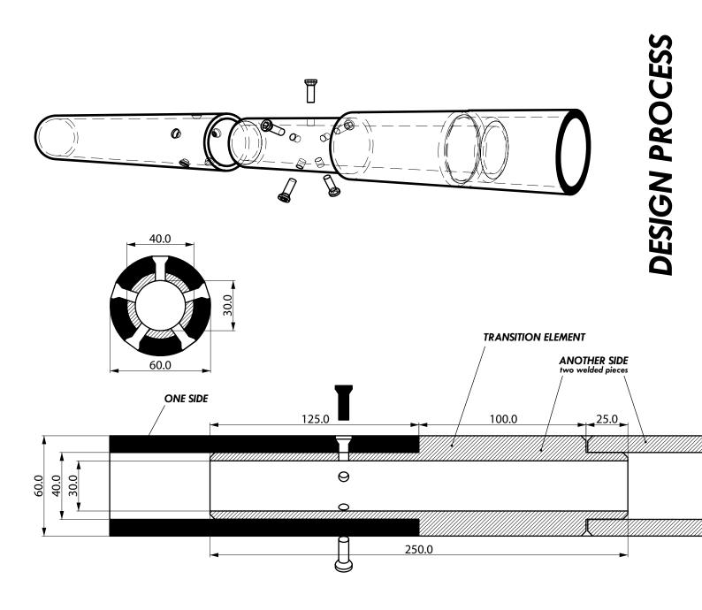
(for example <u>pemat</u> company) that can produce the elements already in right form and necessary length (l=2-2,5m). By complex elements, all pipe parts will be welded together into one piece (drawing SP5).
