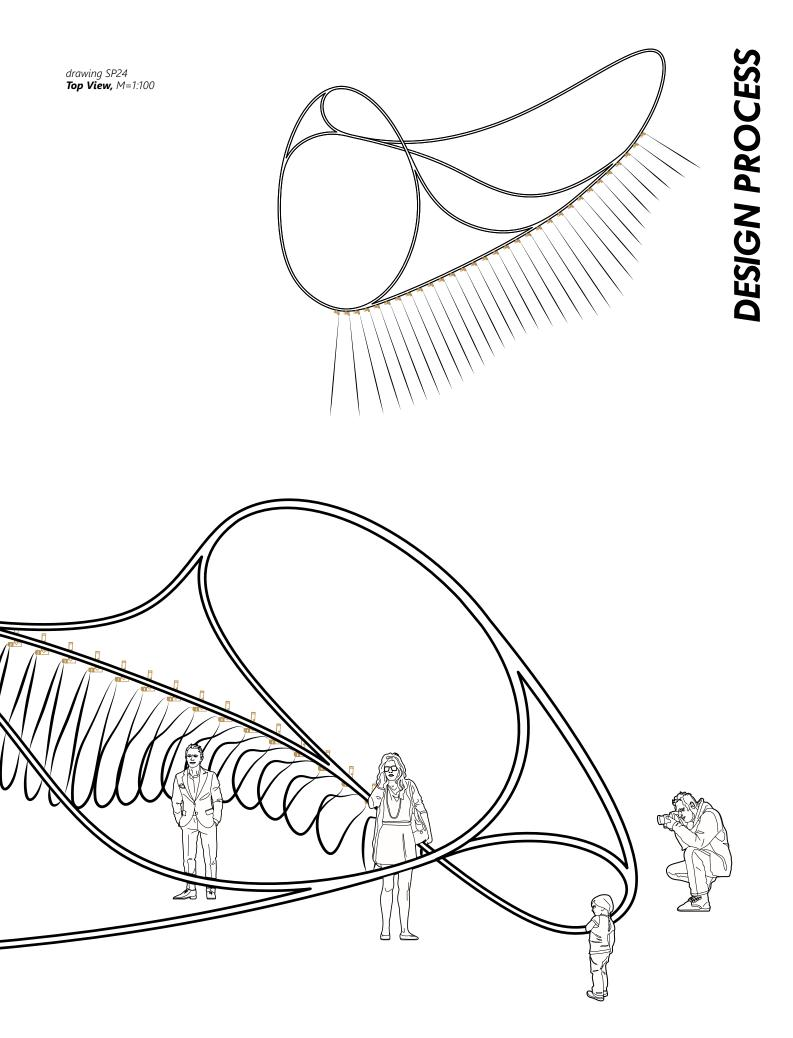
In section **SPACE** was separately discussed and designed two layers of Arcusticon structure: 1. Layerbearing structure and 2. Layer- filling elements.
