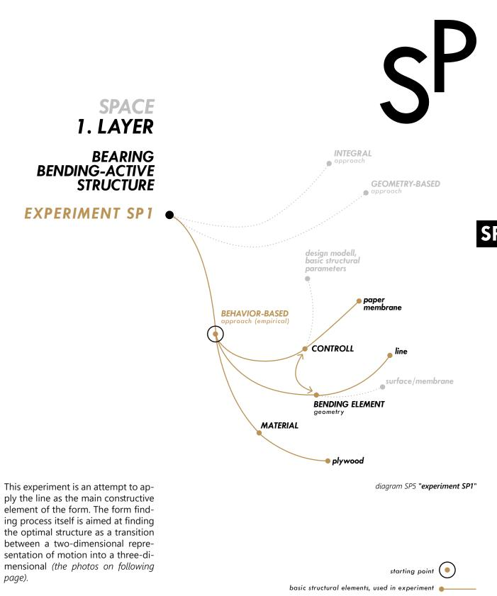
In this experiment, I interpret line through a strip of plywood with a section 2x3mm (bending active material).
