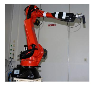
Figure 4.5: COMAU Racer 1.4 equipped with the 6D-force/torque sensor K6-D40. [81]  $\bigodot$  2018 IEEE
