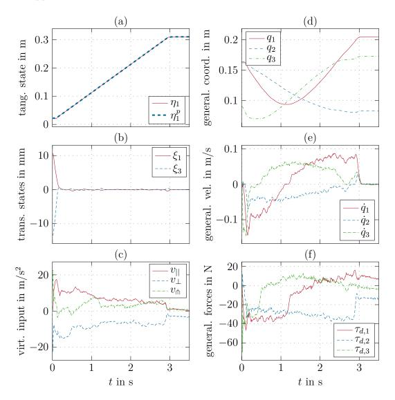
Figure 3.6: Experimental results of the PFC strategy applied to the DELTA robot. [70] © 2017 IEEE
