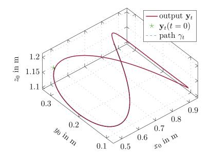
Figure 3.9: Path  $\gamma_t$  and simulated output  $\mathbf{y}_t$  with PFC approach for the 3R elastic joint robot.
