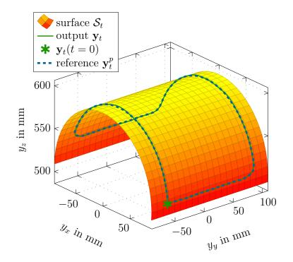
Figure 4.3: Surface  $S_t$  and measured output  $\mathbf{y}_t$  of the SFC experiment on a DELTA robot.
