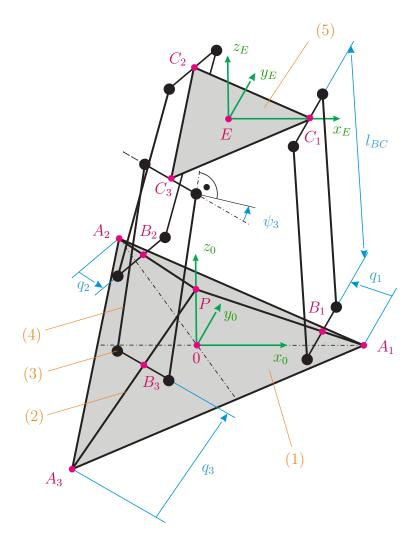
Figure 2.2: Schematic diagram of the DELTA robot FESTO EXPT-45 with linear drives. [70]  $\bigcirc$  2017 IEEE
