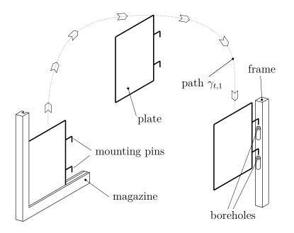
Figure 5.11: Plate mounting using guidance virtual fixtures on a path.
