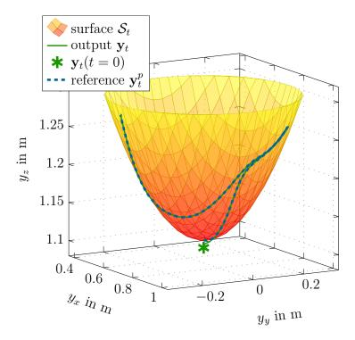
Figure 4.9: Surface  $S_t$  and simulated output  $\mathbf{y}_t$  for the SFC applied to a 3R visco-elastic joint robot.
