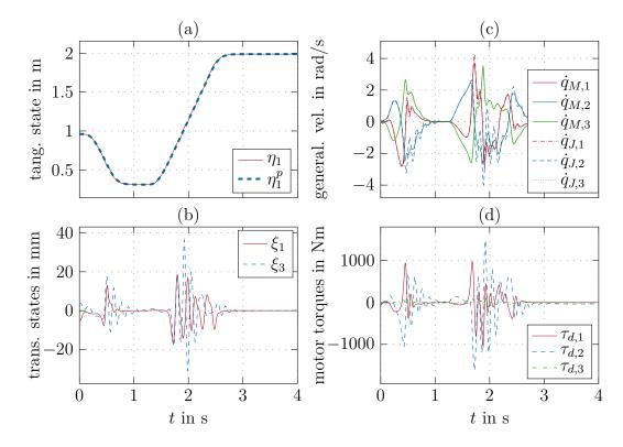
Figure 3.11: Simulated performance of the singular perturbation PFC for a 3R elastic joint robot.
