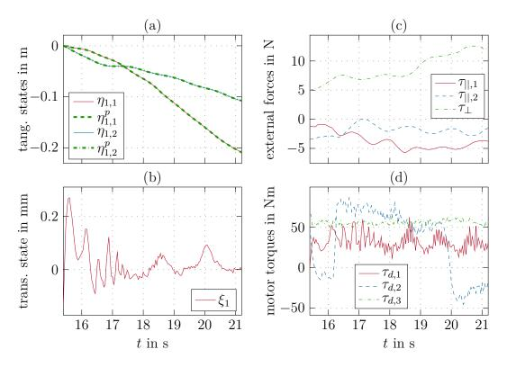
Figure 5.10: Experimental results for forbidden region virtual fixtures for the path segment D in Fig. 5.9 (Example 4). [81] © 2018 IEEE
