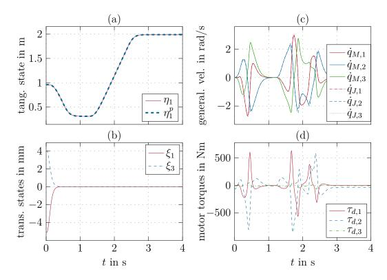
Figure 3.10: Simulated performance of the PFC approach for a 3R elastic joint robot.
