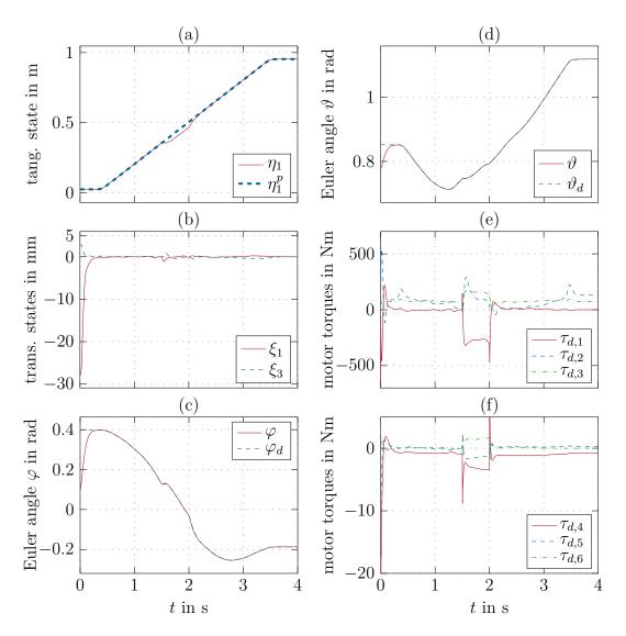
Figure 3.14: Simulated performance of the PFC for a 6R elastic joint robot.
