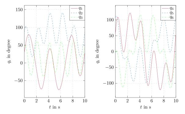
Figure C.1: One period of the optimal excitation trajectory.
