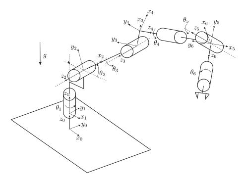
Figure B.1: Coordinate system definition of the COMAU Racer 1.4 for base parameter identification.
