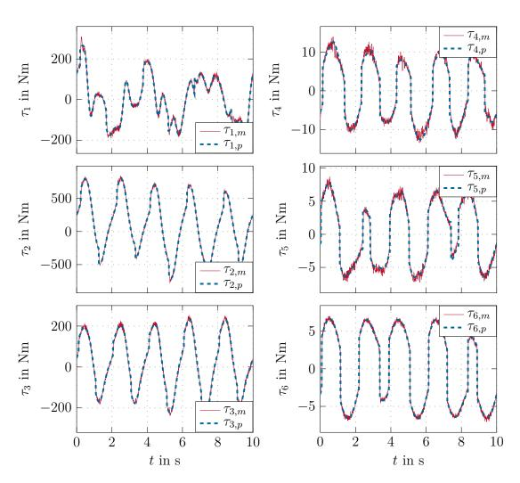
Figure C.2: Measured  $\tau_m$  and predicted  $\tau_p$  torque at the excitation trajectory.
