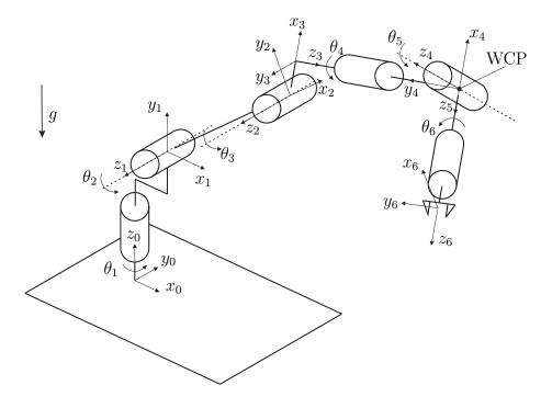
Figure 2.1: Schematic of the COMAU Racer 1.4.
