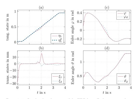
Figure 3.15: Simulated performance of the TTC for a 6R elastic joint robot.
