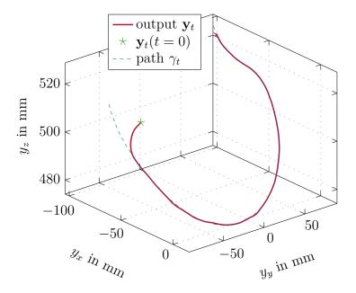
Figure 3.5: Path  $\gamma_t$  and measured output  $\mathbf{y}_t$  of the PFC experiment on a DELTA robot. [70] © 2017 IEEE
