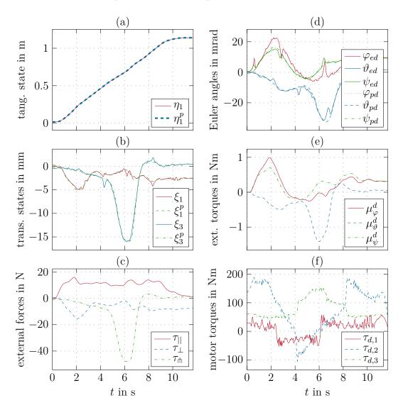
Figure 5.4: Experimental results for soft guidance virtual fixtures (Example 1). [81] © 2018 IEEE
