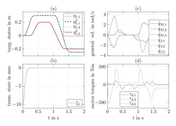
Figure 4.10: Simulated performance of the the SFC approach for a 3R visco-elastic joint robot.
