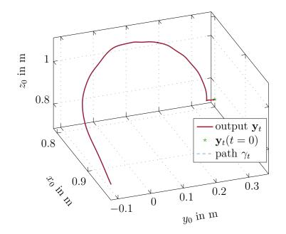
Figure 3.13: Path  $\gamma_t$  and simulated output  $\mathbf{y}_t$  for the 6R elastic joint robot.
