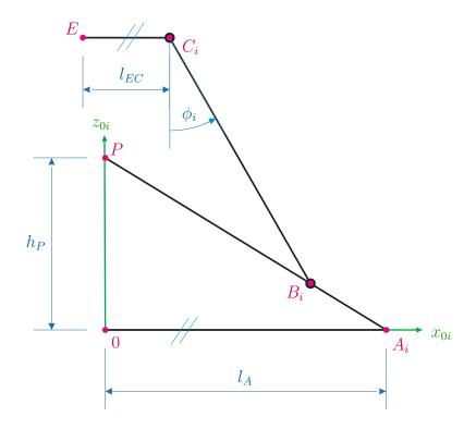
Figure 2.3: Single arm of the DELTA robot FESTO EXPT-45 with linear drives.
