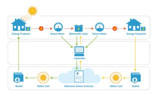
Figure 17. Blockchain P2P Model (using a CSS, Helios). (Based on the Helios Model Overview; loannis, et al. 2017)
