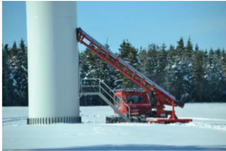
Figure 2.45 Mobile roof built by GDF Suez at Caribou wind parc to access wind turbines requiring maintenance when there is a risk of ice throw, Source: Ice Throwing in Practice, René Cattin, 2011
