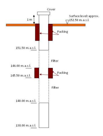
Figure 12 Construction details of LSG39
