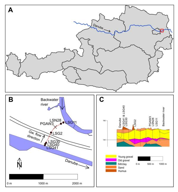
Figure 2 a) Situation of the Natura 2000 protected area (red square) in Austria, b) the sampled transect including monitoring wells LSG41, LSG40, LSG30, LSG2, LSN28 and LSG11. The groundwater abstraction well is depicted as PGAW3 and c) schematic cross section (dotted red line in b) of the transect with the hydrogeological layers and the groundwater monitoring wells (shown as black vertical lines)
