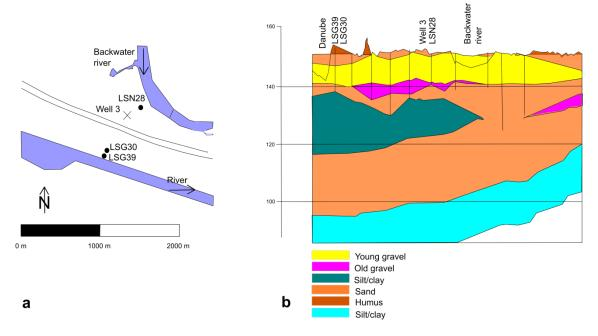
Figure 1 a) Situation of the three sampled groundwater monitoring wells LSG39, LSG30 and LSN28. The groundwater abstraction well is depicted as well 3 and b) schematic cross section of the transect with the hydrogeological layers
