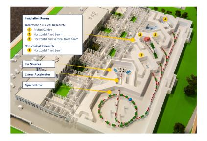
Figure 1.7: Model photo of the accelerator layout (MedAustron 2017)
