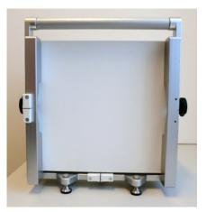
Figure 2.7: RW3 water-equivalent slab phantom from PTW (Freiburg, Germany) (own research)
