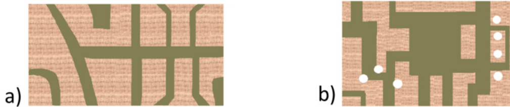
Figure 3.27: Circuit boards of the three interfaces: (a) Interface 1, (b) Interface 2 and Interface 3. The white dots indicate drilled holes.
