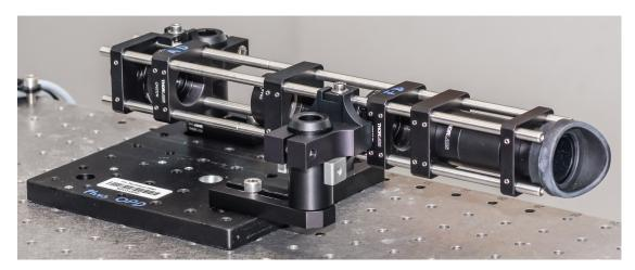
Figure 4.19: The breadboard with the projection optics is mechanically compatible to the breadboard of the MTF-setup. They can easily be exchanged by two mounting screws.
