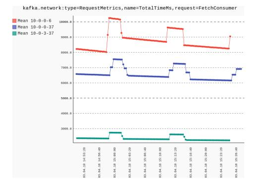
Figure 4.30: Kafka, With Scaling Tool, Fetch Consumer Time, Separated by Host
