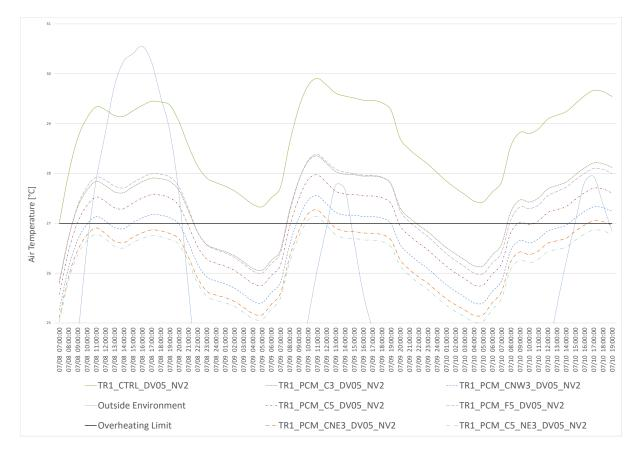
Figure 19: TR1 ventilation strategies & position and quantity simulation cases with the same ventilation pattern on a peak day
