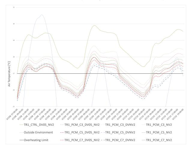
Figure 13: TR1 ventilation strategies scenarios with differing thicknesses; each ventilation scenario is represented with one line type, each thickness with different colour
