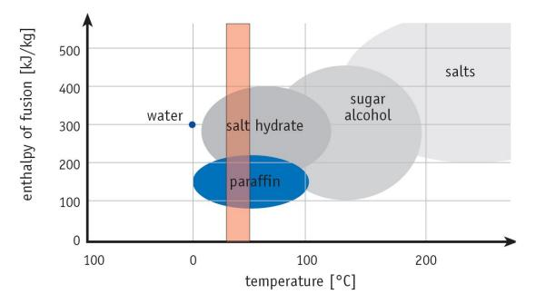
Figure 1: Temperature ranges and corresponding enthalpy of fusion of several PCMs. Red zone indicates the acceptable temperature ranges for residential usage.
