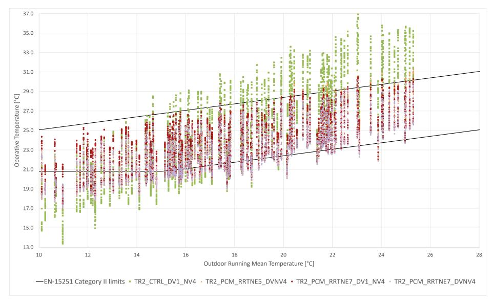
Figure 22: EN-15251 Adaptive comfort category II acceptability limits for best performing TR2 position and quantity scenarios
