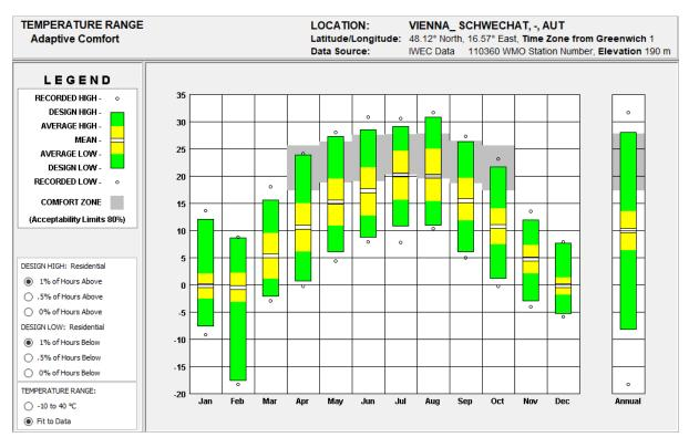
Figure 6: Overview of the IWEC standard weather file
