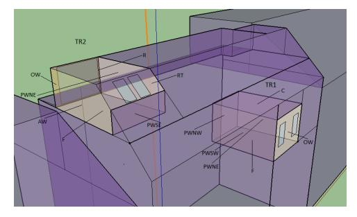
Figure 8: Test rooms and respective surfaces
