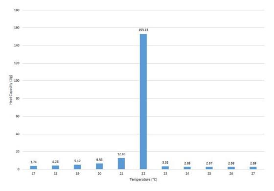
Figure 3: PureTemp 25 Heat Capacity Solidification Histogram
