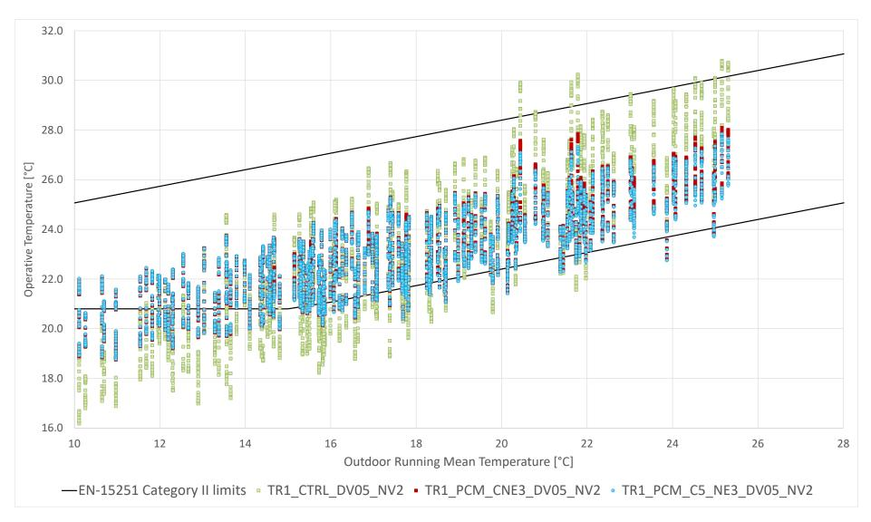
Figure 20: EN-15251 Adaptive comfort category II acceptability limits for best performing TR1 position and quantity scenarios
