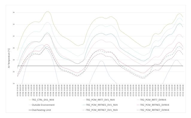
Figure 21: TR2 ventilation strategies & position and quantity simulation cases with same ventilation patterns on a peak day
