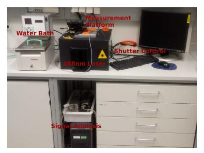
Figure 11: Light scatter station set-up
