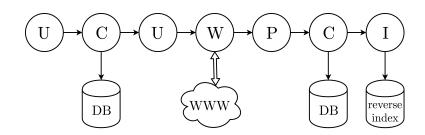
**Figure 2.** The indexing pipeline: The Updater (U) uses the CatalogStore's (C) metadata to determine feeds that require updating  $(U \rightarrow C \rightarrow U)$ . The Web Crawler (W) loads the XML from the web, the Parser (P) transforms the feed data to domain objects. The CatalogStore persists the data and forwards selected metadata to the IndexStore (I)
