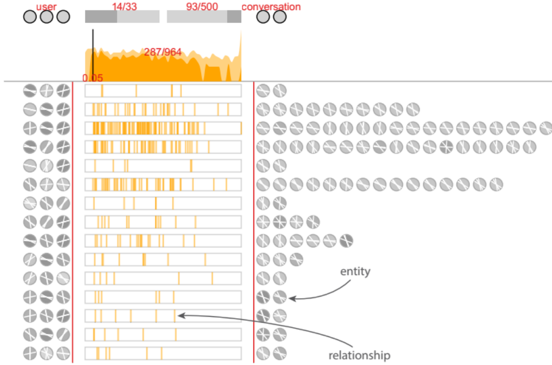
Figure 3.13: User interface of BiDots . Rows represent biclusters, circles represent unique entities and orange line strips represent weighted relationships between entities [ZSCC18].
