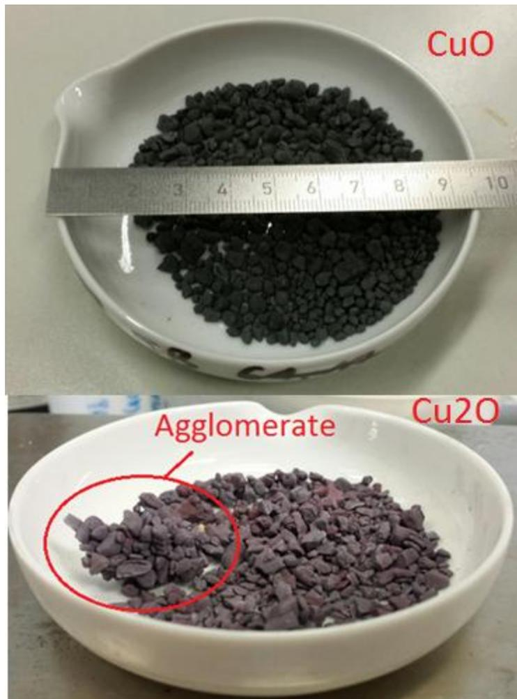
Figure 39: Copper oxide in the oxidized/discharged (top) and reduced/charged (bottom) state
