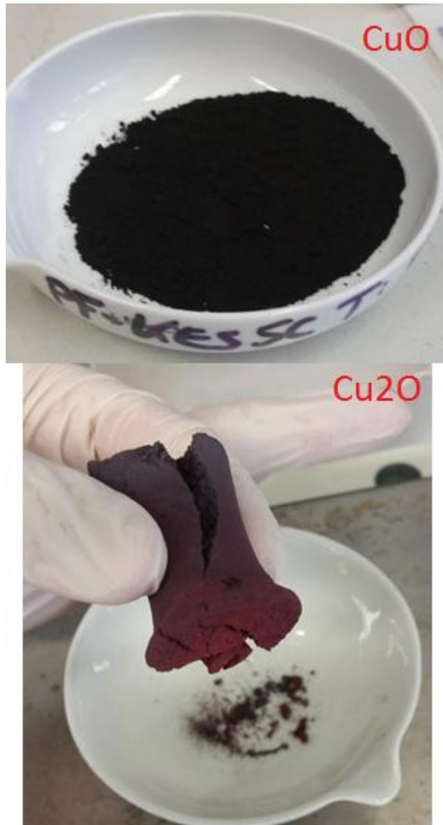
Figure 40: Copper oxide fine discharged powder (top) and charged solid block (bottom)
