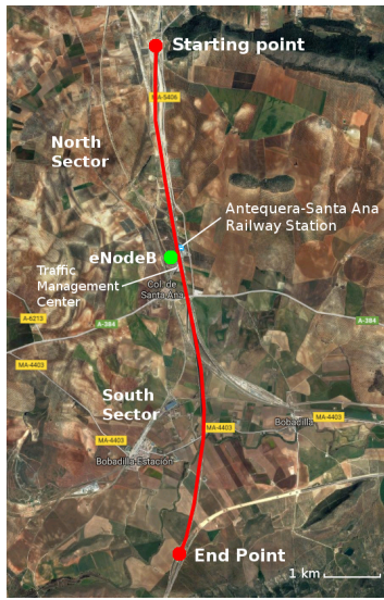
(a) Map of the measurement environment - BS position indicated with a green dot.
