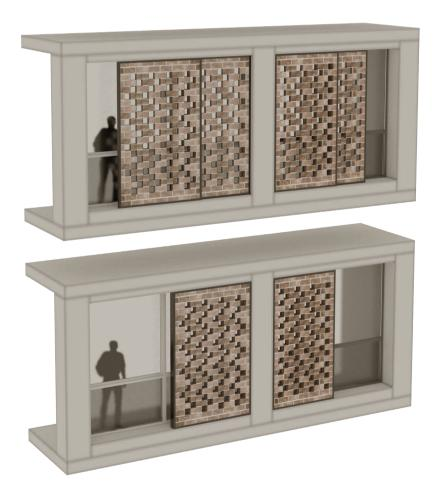
Fig. 5.11: The function of the sliding clay brick panels
