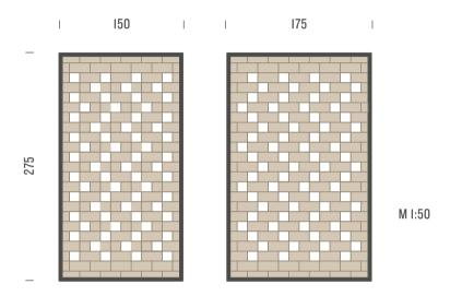
Fig. 5.10: Front view of the brick panels
