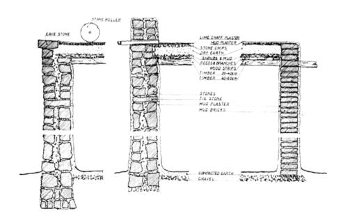
Fig. 5.20: Detailed drawing for a traditional stone and mud brick wall with flat roof
