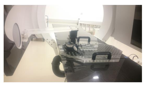
Figure 5.1: Experimental setup of the focal spot measurements: the X-ray head on the left side was placed in a horizontal position, with the slit camera directly next to the exit window. The detector was positioned parallel.
