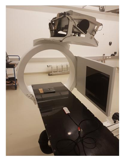
Figure 4.1: Experimental setup of  $HVL_{A1}$  measurements. The NOMEX Multimeter was placed on the patient couch, in the central beam of the X-ray source.
