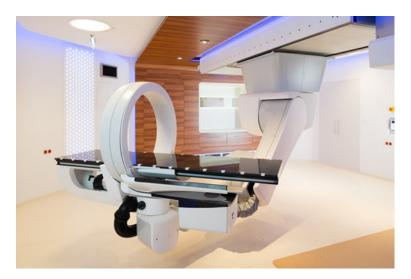
Figure 2.1: ImagingRing<sup>™</sup> System at MedAustron (from [43]) The ring sourrounds the patient couch. Both are mounted on a robotic arm. X-ray head and detector are positioned underneath the patient couch.
