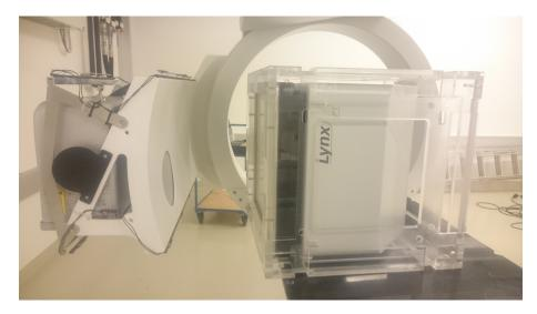
Figure 6.1: Experimental setup of heel measurements. Left: the X-ray head of the ImagingRing<sup>™</sup> System, Right: The Lynx camera. The detector (not in the picture) of the ImagingRing<sup>™</sup> System was moved to the top in order to protect the electronics from unfiltered radiation.
