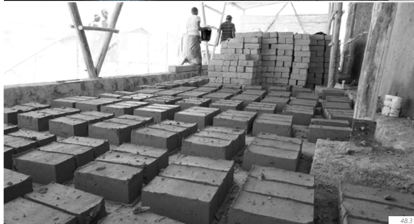
fig. 48.3 | predrying of bricks under the shed roof
