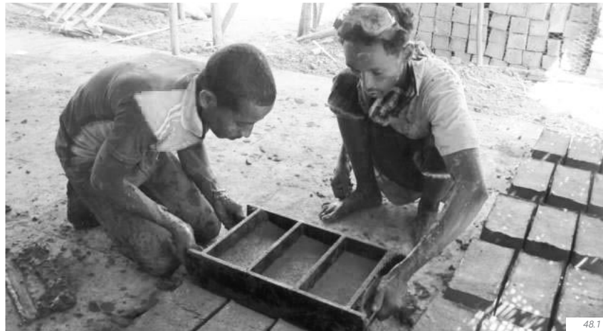
fig. 48.1 | brick production process – removing the mould right after pulling the overspill material off and straightening the top surface
