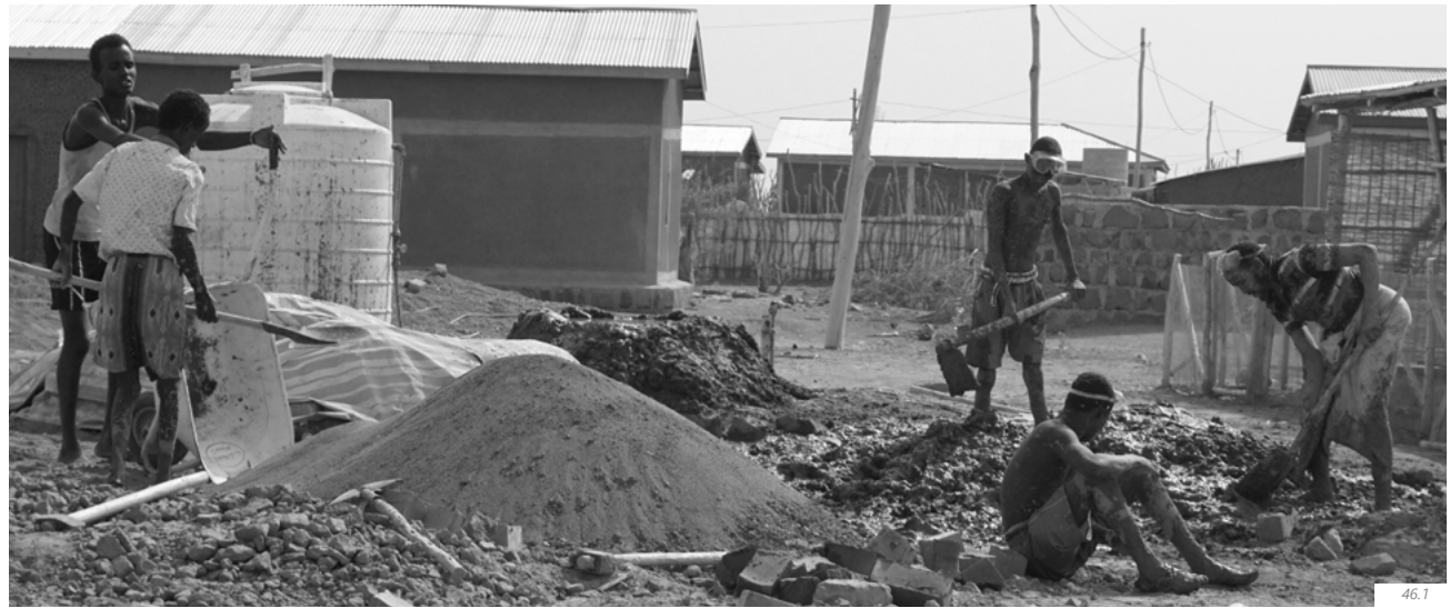
fig. 46.1 | preparing the raw material for bricks production – on the left: preparing a new pile of the composition and mixing it dry first – in the background: an already finished prepared pile with a hollow on top to fill it with water and let it soak for two days – on the right: mixing the already soaked material again and add water to get the right texture for production
