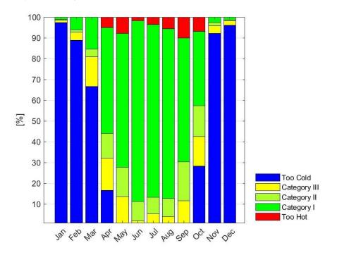
Figure 17: Evaluation of indoor temperatures according to thermal categories, BC, thermal self-sufficiency 56%
