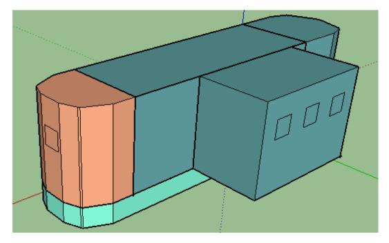
Figure 10: Zoning for simulation in EnergyPlus
