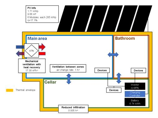
Figure 12: Representation of Case 2 ventilation and infiltration
