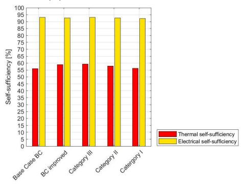
Figure 20: Self-sufficiency depending on air-tightness and ventilation rates
