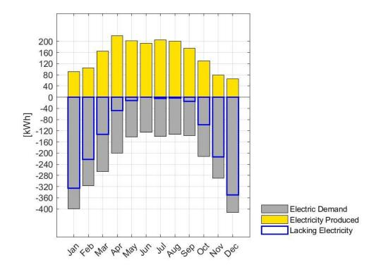
Figure 21: Electric demand, production, and shortage of electricity per month, C3, electrical self-sufficiency 49%
