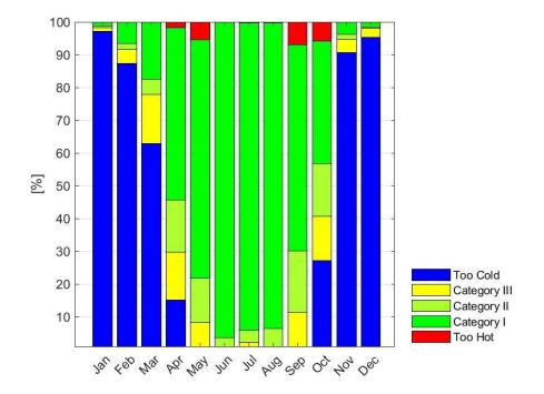
Figure 19: Evaluation of indoor temperatures according to thermal categories, C2, thermal self-sufficiency 59%
