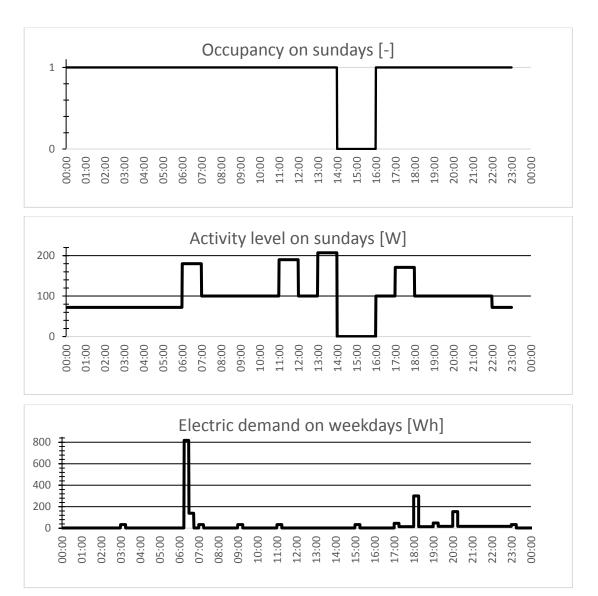
This graph includes all electrical equipment including lighting, hot water equipment but no heating equipment.
