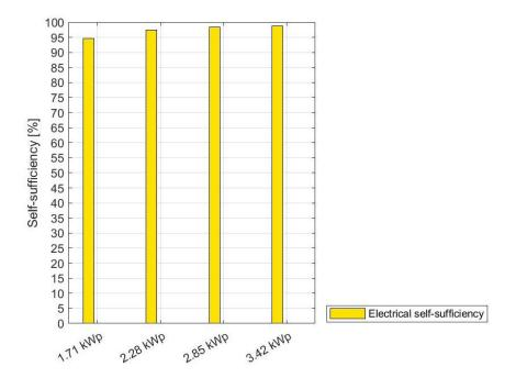
Figure 26: Electrical self-sufficiency dependent on photovoltaic size with a battery storage of 10.06 kWh
