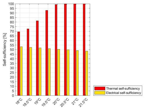
Figure 23: Self-sufficiency as a function of the heating setpoint
