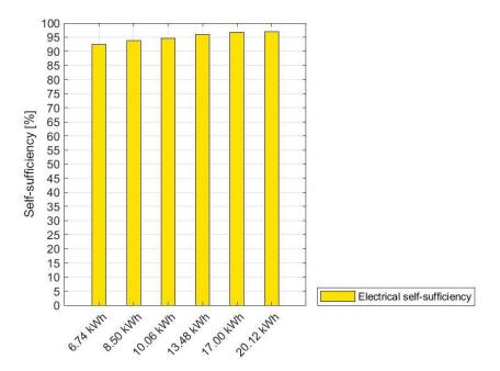
Figure 24: Electrical self-sufficiency dependent on electrical storage size
