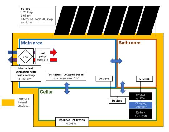
Figure 13: Representation of Case 3 heating system
