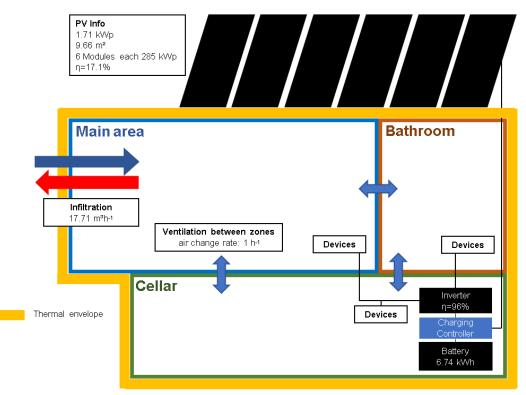
Figure 11: Representation of the Base Case system set-up
