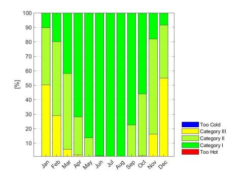
Figure 22: Evaluation of indoor temperatures according to thermal categories, C3, thermal self-sufficiency 100%
