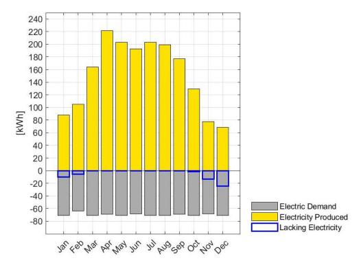
Figure 15: Electric demand, production, and shortage of electricity per month, BC, electrical self-sufficiency of 93%
