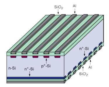
Figure 16: Double sided silicon strip detector [21]
