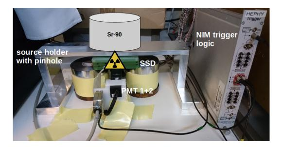
Figure 41: Module testing with Sr-90
