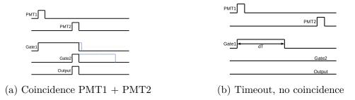
Figure 28: Asynchronous coincidence [31]
