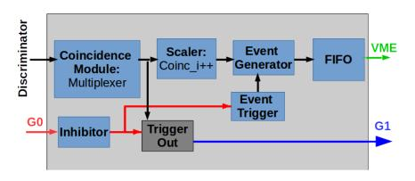
Figure 26: COSCAT FPGA design, G0, G1 are LEMO I/O ports
