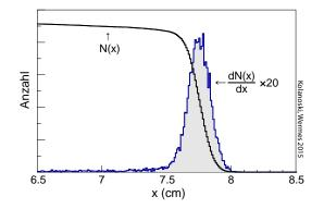
Figure 3: Geant4 Simulation of 100 MeV protons travelling through water [6]
