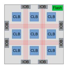
Figure 22: Schematic drawing of a FPGA with configurabel logic blocks (CLB), interconnect wires, I/O blocks (IOB) and a flash memory for the circuit design.
