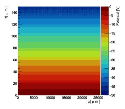
Figure 52: Calculated potential of the whole detector, p-side
