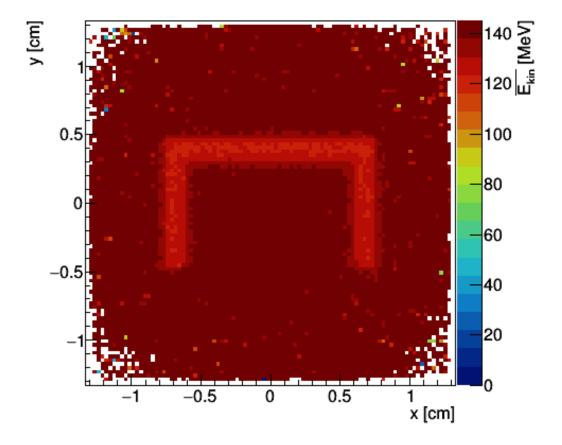
Figure 69: LEGO brick, proton computed radiography, 145.4 MeV
