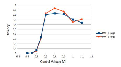
Figure 46: Plateau curve of the bigger PMTs
