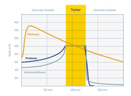
Figure 1: Depth-dose profile of photons vs. ions [1]
