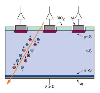
Figure 15: Cross secrion of a single-sided Si-strip detector [21]
