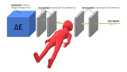
Figure 4: Setup of a proton computed tomography
