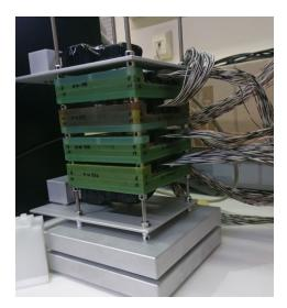
Figure 42: Telescope testing with cosmic myons
