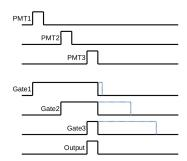
Figure 29: Coincidence PMT1 + PMT2 + PMT3 [31]
