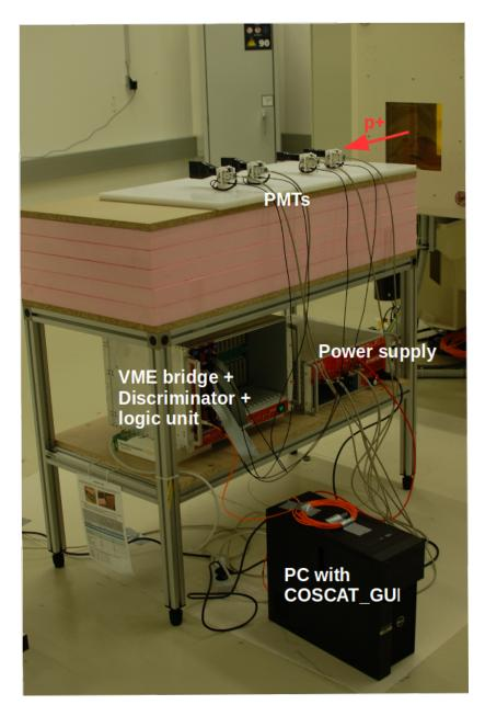
Figure 32: Plateau curve measurement setup [38]
