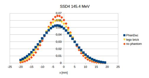
Figure 65: Fitted beam profiles for different phantoms at SSD4
