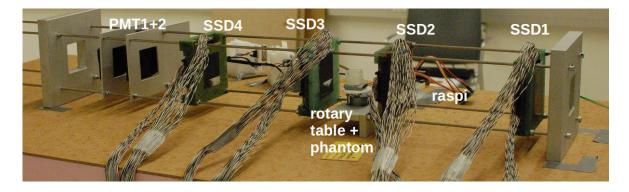
Figure 43: Beam telescope setup at MedAustron [31]
