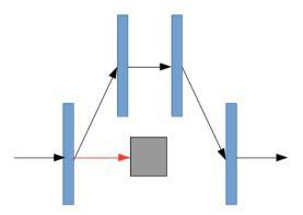
Figure 20: 4 chopper magnets (blue) with a beam dump (grey)
