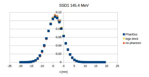
Figure 64: Fitted beam profiles for different phantoms at SSD1
