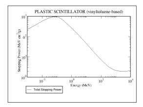
Figure 2: Total stopping power for protons in plastic scintillators [7]
