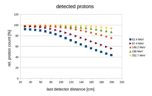
Figure 55: Beam telescope length without a scintillator in front
