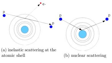
Figure 5: Interaction of protons with matter
