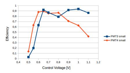
Figure 47: Plateau curve of the smaller PMTs
