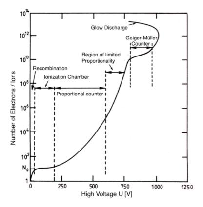
Figure 12: Different operational modes of a gaseous detector [20]
