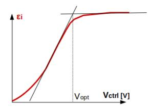
Figure 31: Plateau curve of a PMT
