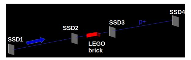
Figure 40: Geant4 simulation of a pCT setup
