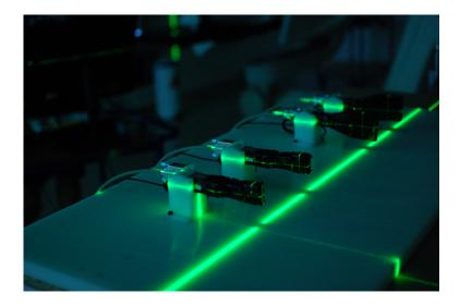
Figure 33: Alignment of all four scintillators [38]
