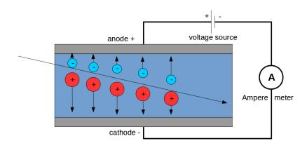
Figure 11: Operation principle of a gaseous detector
