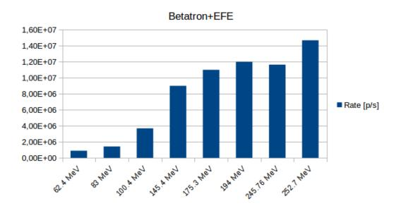
Figure 51: Energy dependence of the Betatron+EFE method
