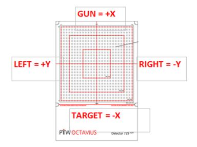
Figure 34: Octavius ionization chamber array [39]
