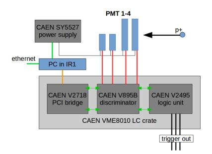
Figure 23: Particle counting and trigger setup
