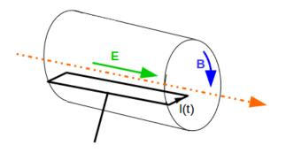
Figure 21: Schematic drawing of a betatron
