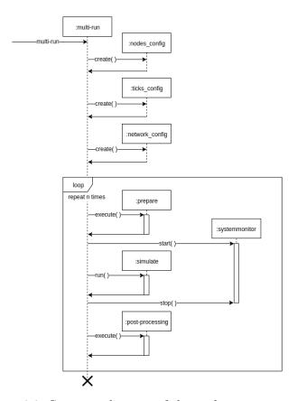
Figure 3.2: Sequence diagram of the multi-run command
