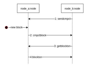
Figure 8.1: Compact block relay mechanism [bip]
