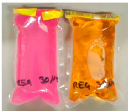
Fig. B 8. Example of a low-cost E. coli assay using Resorufin \beta -D-Glucuronide 19
