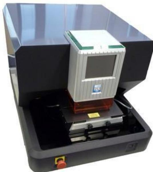
Figure 3.2: New Wave 213 laser ablation device employed for the performed experiments
