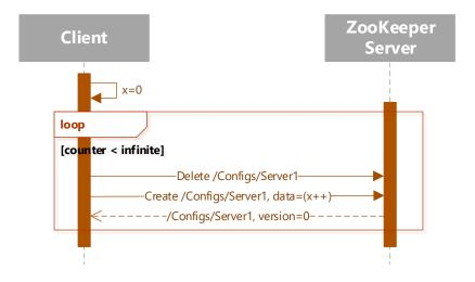
Figure 4.4: An example of a failure in conditional execution. The znode data is updated infinitely, but the version number remains the same.
