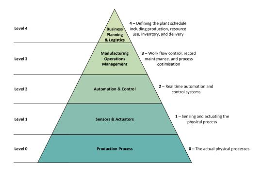
Figure 1.2: The five layers of the automation pyramid [23].
