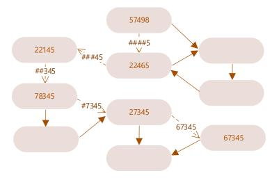
Figure 3.4: An example of Plaxton-based mesh routing in Tapestry.
