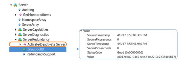
Figure 4.10: The "GroupGUID" variable node and "Activate/Deactivate Server" method node in the OPC UA address space.
