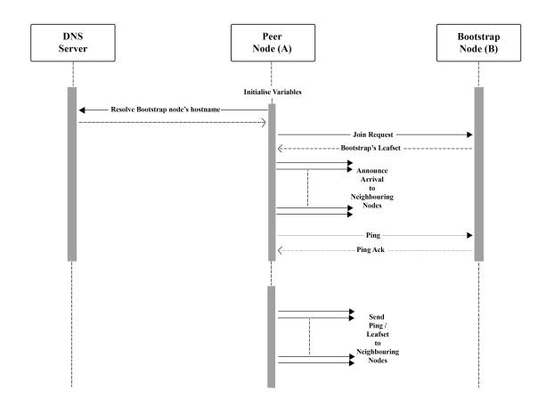
Figure 3.17: The operational mechanisms of the vanilla Chimera P2P protocol.
