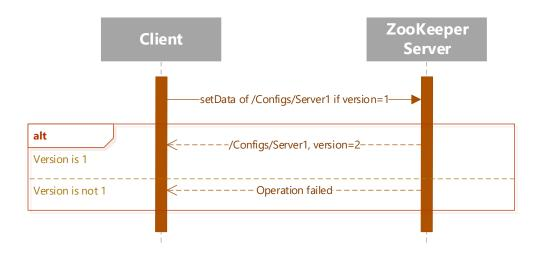
Figure 4.3: The coordination of concurrent updates using conditional execution. A data setting operation is dependent on znode */Configs/Server1* having a version number of 1. If the data set operation succeeds, the znode's version number is incremented to 2.
