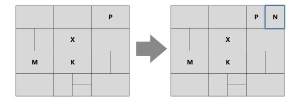
Figure 3.5: A 2D CAN network showing a split of zone P to accommodate a newly joined node N.
