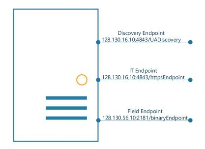
Figure 2.7: An example device with discovery, OPC UA HTTPS, and OPC UA TCP endpoints.
