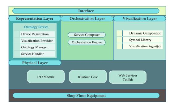
Figure 2.4: The eScop system architecture [45].
