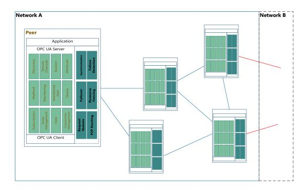
Figure 5.1: The main building blocks of the service overlays for resilient CPPS.
