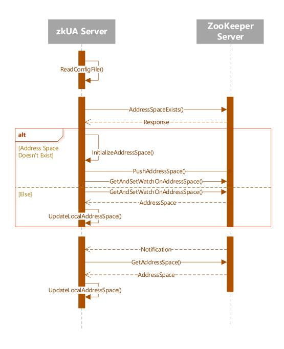
Figure 4.12: A UML sequence diagram showing the interactions taking place between a zkUA Server and ZooKeeper. The triggered notification implies that the address space stored on ZooKeeper was manipulated by a zkUA Server.
