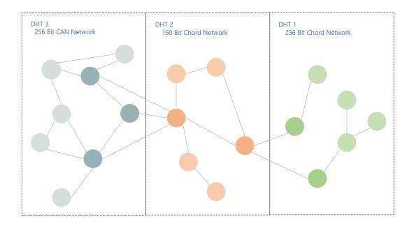
Figure 3.14: An example of three bridged DHTs for inter-system routing as adapted from [177].
