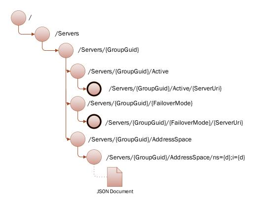
Figure 4.9: The hierarchical ZooKeeper data model for OPC UA servers redundancy.
