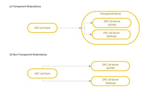
Figure 4.7: a) Transparent and b) non-transparent redundancy in OPC UA [133].
