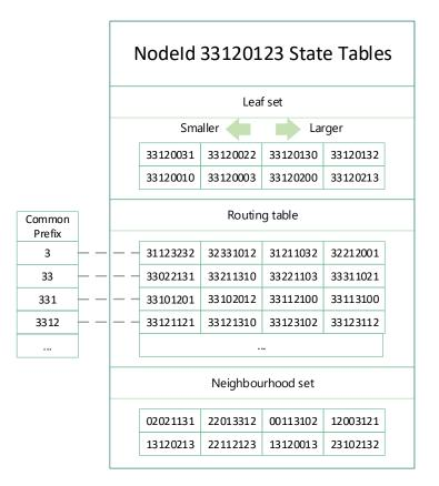
Figure 3.6: Pastry leaf set, routing table, and neighbourhood set. The host node has a node ID 33120123, b = 2, and l = 8. All IDs are in  $base = 2^{b} = 4$ . Each row n in the routing table shares n digits with the host node.
