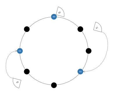
Figure 3.3: A chord ring with m=3, 3 nodes, and 3 keys. Keys K1 and K5 are located at nodes N3 and N6 as they are the successors to nodes N1 and N5, respectively.
