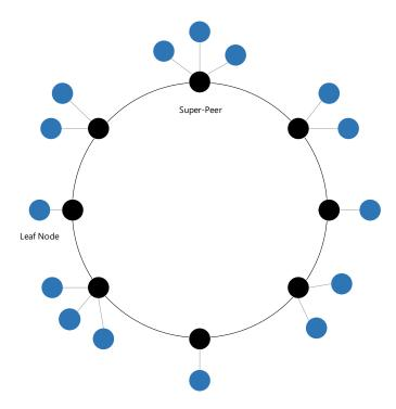
Figure 3.13: An example of a two-layer network in [174] with a Chord network upper layer and star-shaped connections with lower layer leaf nodes.
