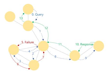
Figure 3.8: A request lookup in the Freenet network. A failure is returned in step 5 to break a routing loop causing the request to be forwarded down an alternate path in step 8.
