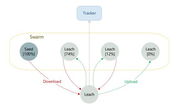
Figure 3.9: An example BitTorrent system. A new leach contacts the tracker to receive a list of peers from the tracked swarm. The leach connects to the swarm and downloads/uploads pieces of the shared file(s).
