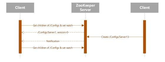
Figure 4.5: An example of a watch and notification on ZooKeeper. The watch set on the /Configs znode by the first client (left) is triggered by the creation of a new child znode under the same path by the second client (right).
