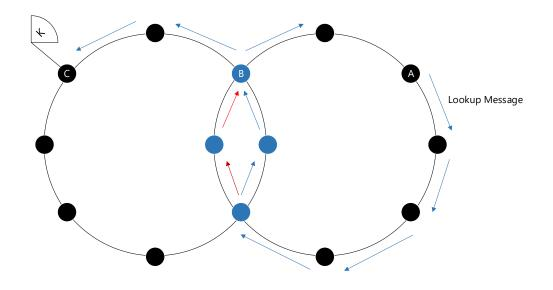
Figure 3.15: An example of Babelchord lookup routing in two floors as adapted from [178]. Node A queries for resource K on node C. The lookup from node A reaches node B twice. The query following the red path is terminated at node B as it has already been processed by node B via the blue path.
