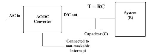
Figure 3.24: A mechanism for detecting and delaying the loss of input power.
