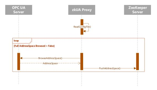
Figure 4.11: A UML sequence diagram showing the actions of a zkUA Proxy component.
