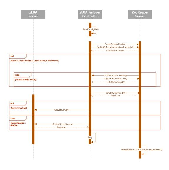
Figure 4.13: A UML sequence diagram showing the interactions taking place between a zkUA Server, a zkUA FC, and ZooKeeper.
