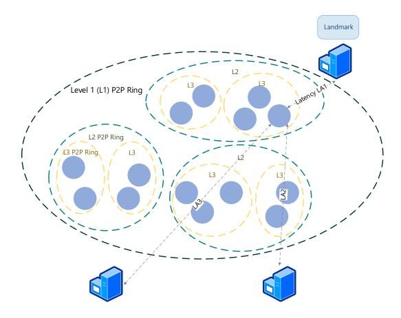
Figure 3.11: An example of a three level HIERAS network hierarchy.
