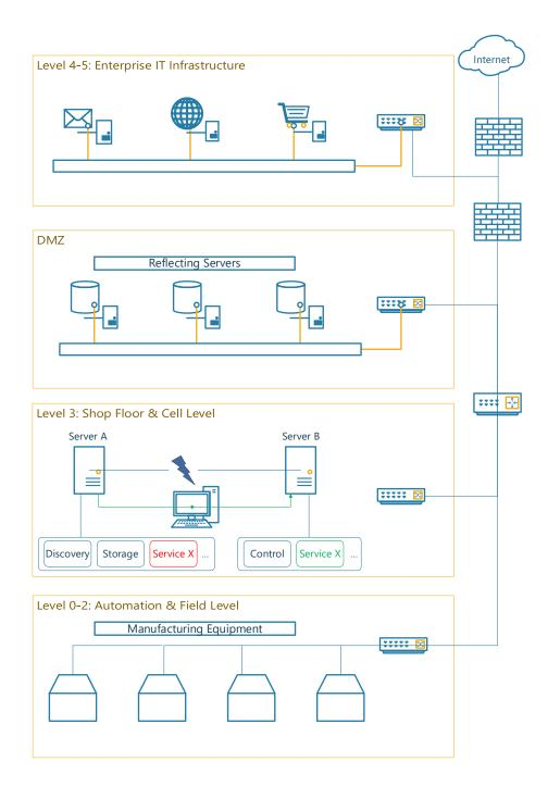
Figure 1.3: The envisioned resilient and robust SO manufacturing infrastructure. Service X on server A fails and is replicated on a different server (server B). With the link to the new service down, requests are re-routed through existing infrastructure to establish a new path for the continuity of data exchange.
