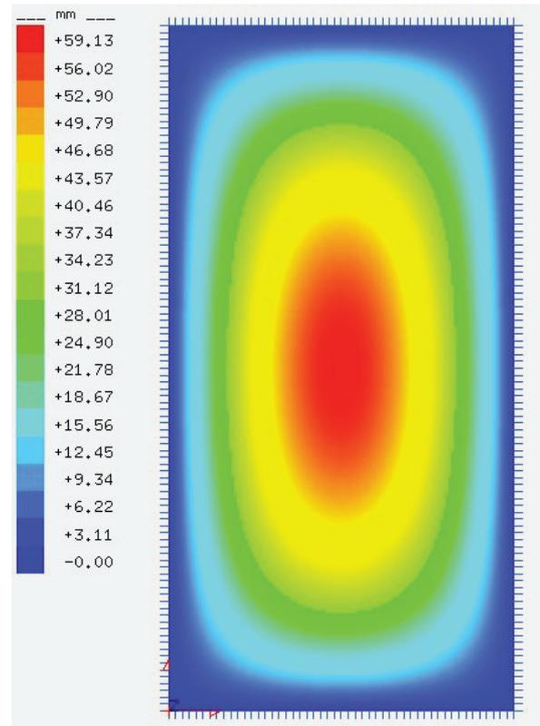
Fig. 4.6: FE-analysis of the pane under 2.30 kN/m<sup>2</sup> load – deflections
