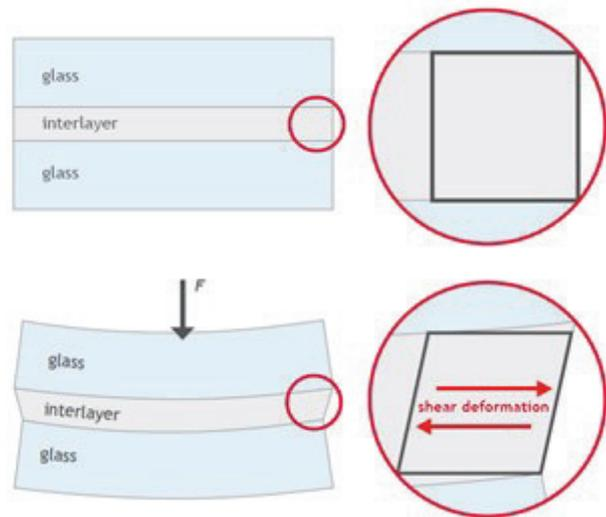
Fig. 4.9: Laminate under bending [56]
