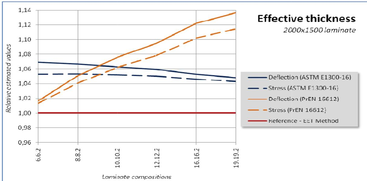
Fig. 6.3: Estimated effective thickness values relative to the results of the EET-method for various compositions – Laminate size 2000x1500 mm
