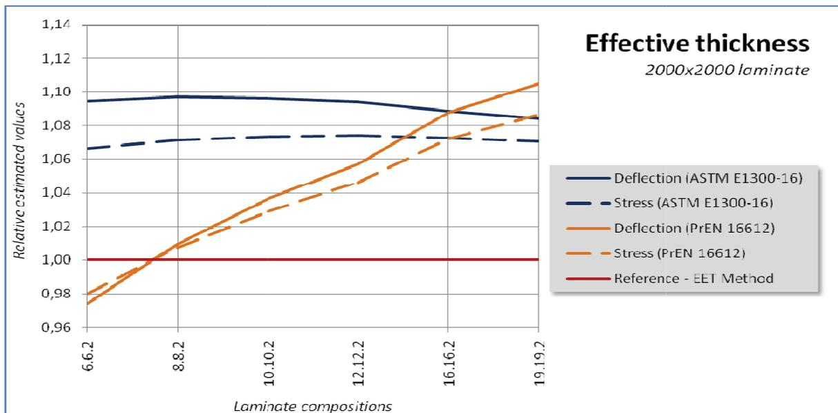
Fig. 6.4: Estimated effective thickness values relative to the results of the EET-method for various compositions – Laminate size 2000 x 2000 mm
