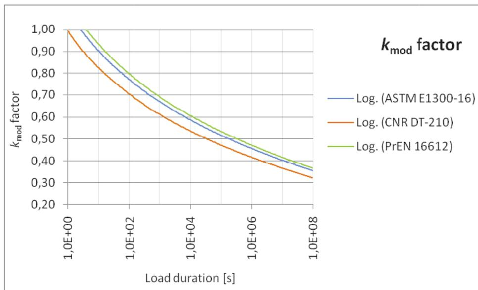
Fig. 4.7: Comparison of the values of the  $k_{\text{mod}}$  factor estimated with different formulas
