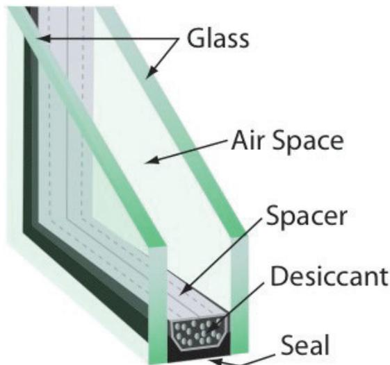
Fig. 4.13: Composition of a simple insulating unit [48]
