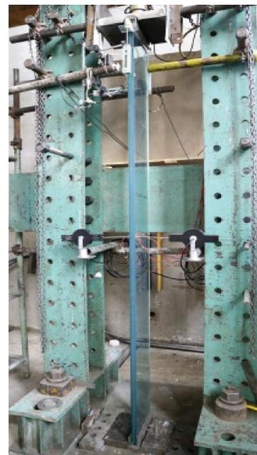
Fig. 5.2: Test set-up: Laminate under axial compression [36]
