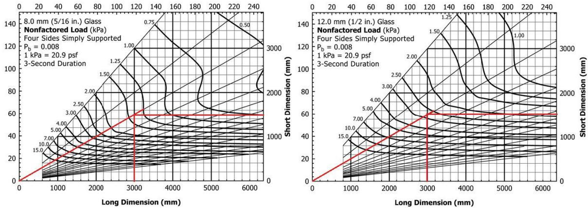
Fig. 6.6: Charts for 8 mm and 12 mm thick glass plies ([2], A1.8 and A1.10)
