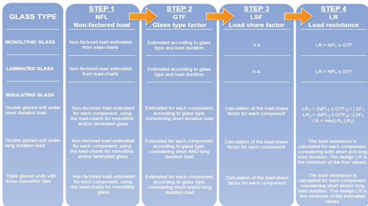
Fig. 4.2: Flow chart of the verification procedure with glass charts (Self-made fig. based on [2])
