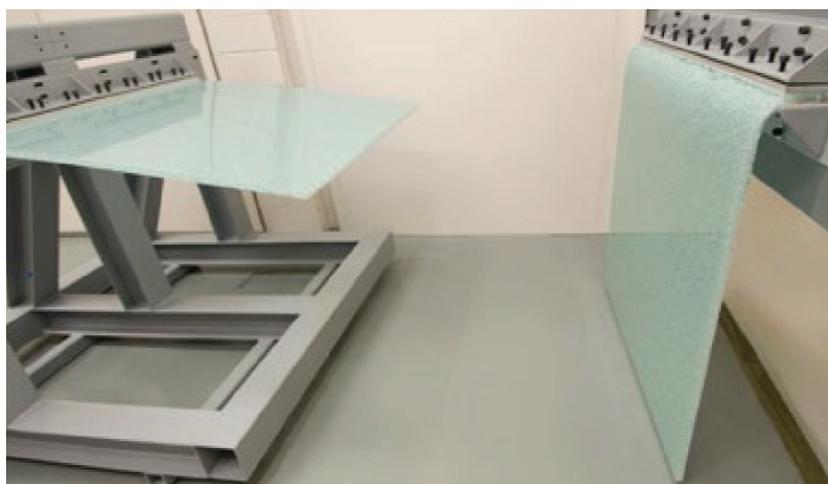
Fig. 4.10: Post-breakage behaviour of cantilevering laminates with SentryGlas (left) and PVB interlayer (right) [57]
