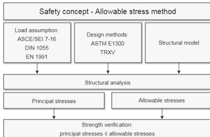
Fig. 4.1: General procedure for strength verification, based on the allowable stress method (Self-made fig. based on [40])
