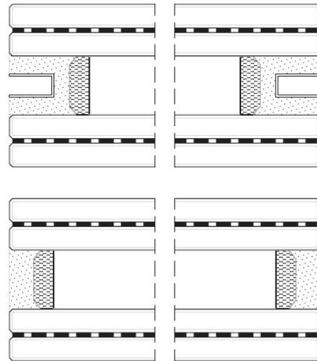
Fig. 4.14: Sections of insulating units with spacer (bottom) and additional C-channel for mechanical fixing (top) – Self-made fig.
