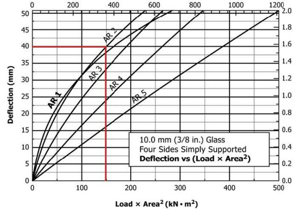
Fig. 4.4: Deflection chart for a 10 mm thick monolithic glass lite [2]
