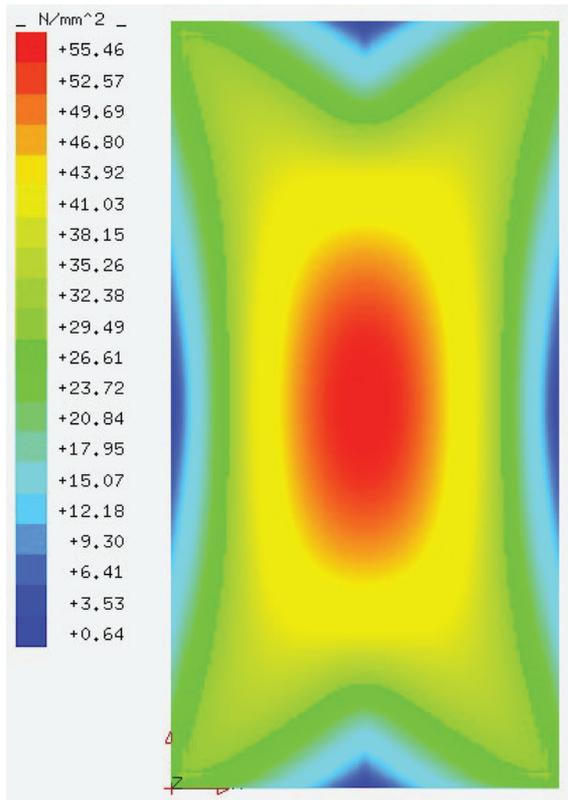
Fig. 4.5: FE-analysis of the pane under 2.30 kN/m<sup>2</sup> load – principal stresses
