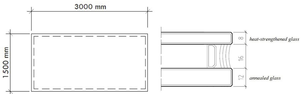
Fig. 6.5: Double glazed insulating unit
