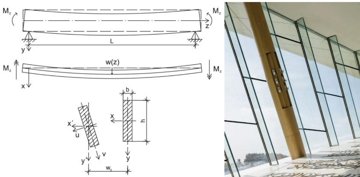
Fig. 5.3: Flexural-torsional deformation of a beam element under bending – Self-made fig. based on [3]
