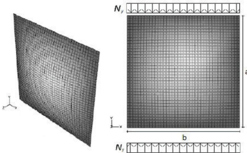
Fig. 5.5: Panel simply supported along the edges subjected to in-plane compression – Self-made fig. based on [3]
