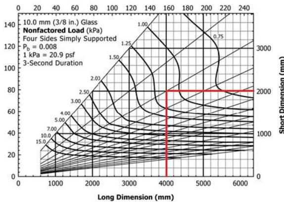
Fig. 4.3: NFL chart for a 10 mm thick monolithic glass lite [2]
