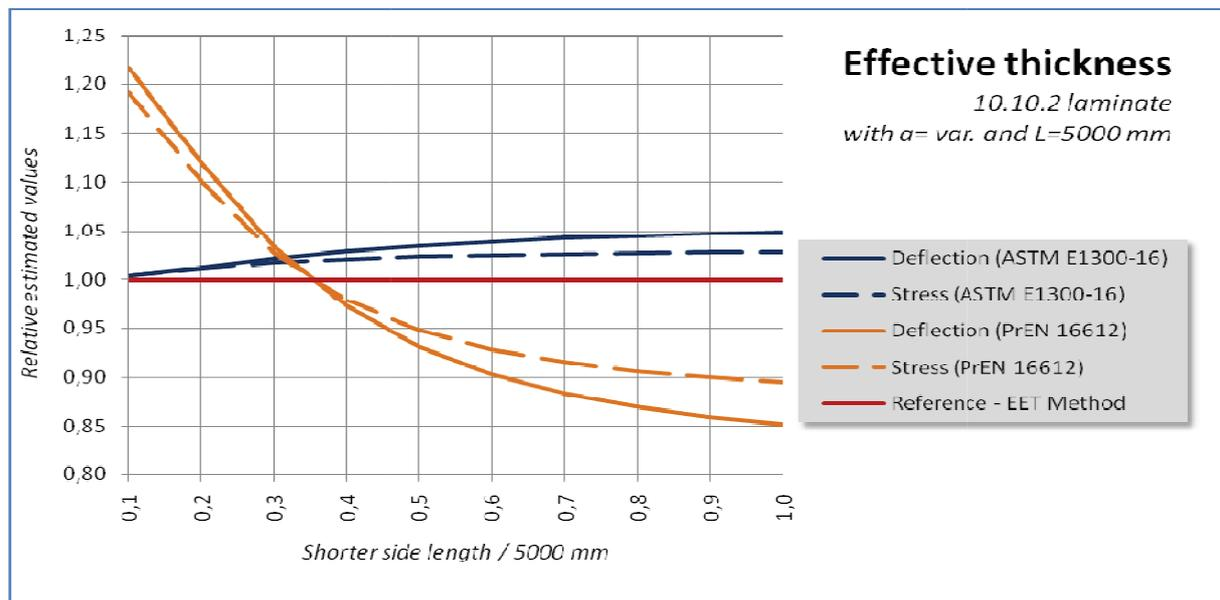
Fig. 6.2: Estimated effective thickness values relative to the results of the EET-method for a 10.10.2 laminate with various side dimensions
