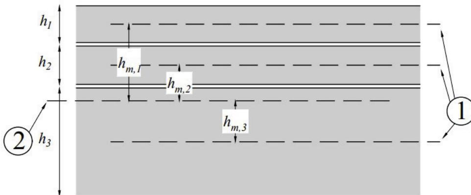
Fig. 4.12: Laminated glass thickness dimensions.
