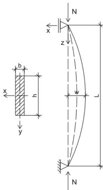
Fig. 5.1: Deflected shape of an Euler-beam under axial loading - Self-made fig. based on [3]
