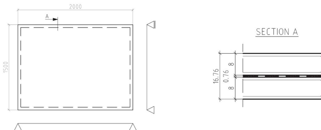
Fig. 6.1: Overview of the exemplary glazing element
