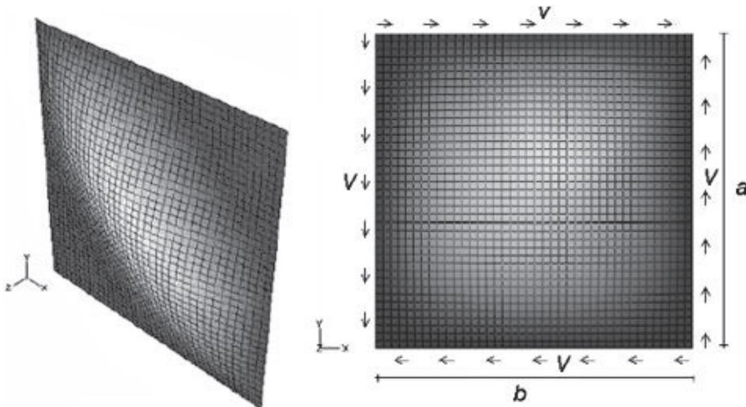
Fig. 5.6: Panel supported along its edges and subjected to in-plane shear forces – Self-made fig. based on [3]
