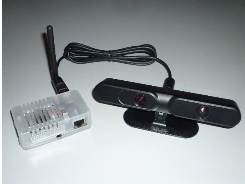
Figure 3.1: The two hardware components of the fearless system: single-board computer (left), depth sensor (right)
