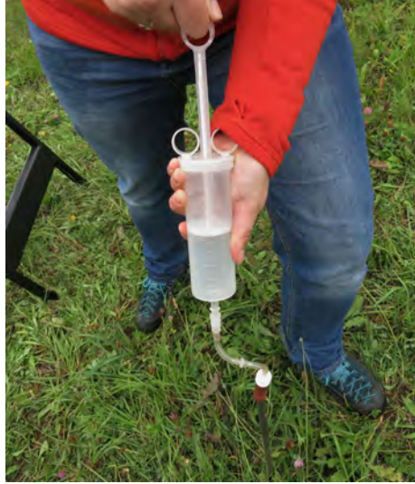
Figure 6.3.: Taking a soil gas sample using a syringe.
