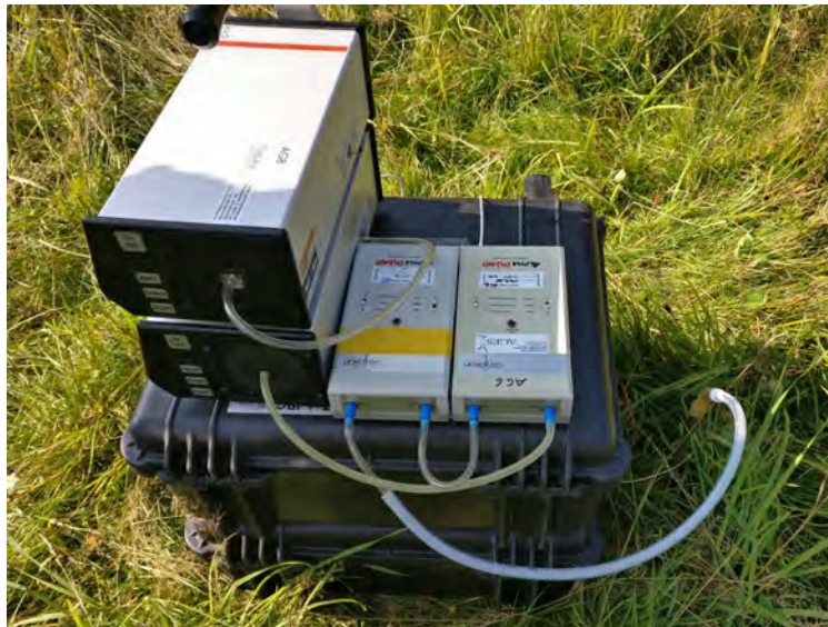
Figure 6.4.: Photograph of the setup to measure the activity concentration of radon and thoron in soil gas.
