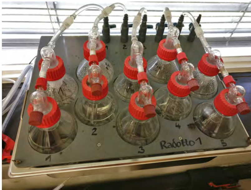
Figure 5.6.: Photograph of the radon source RADOTTO 1.
