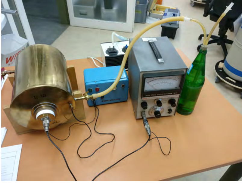
Figure 7.1.: Photograph of the setup to measure the radon activity concentration in a water sample.
