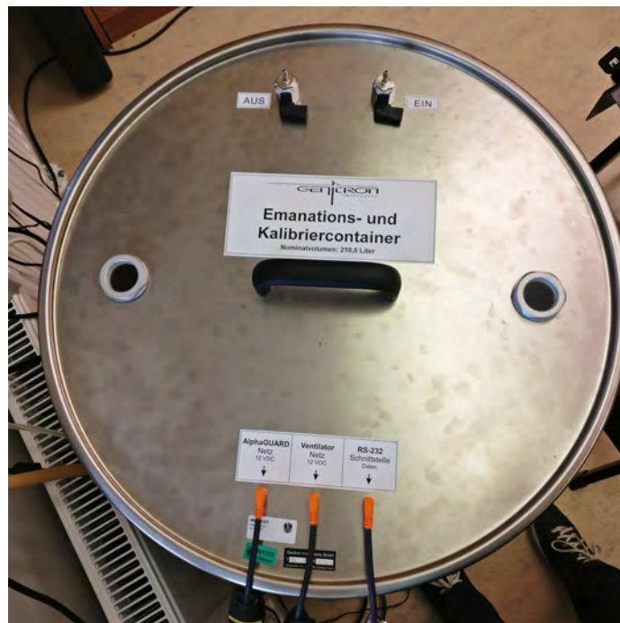
Figure 5.4.: Photograph of the emanation and calibration container.
