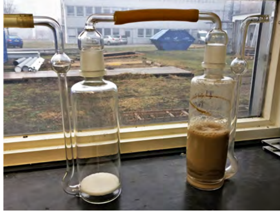
Figure 5.8.: Photograph of the thoron source.
