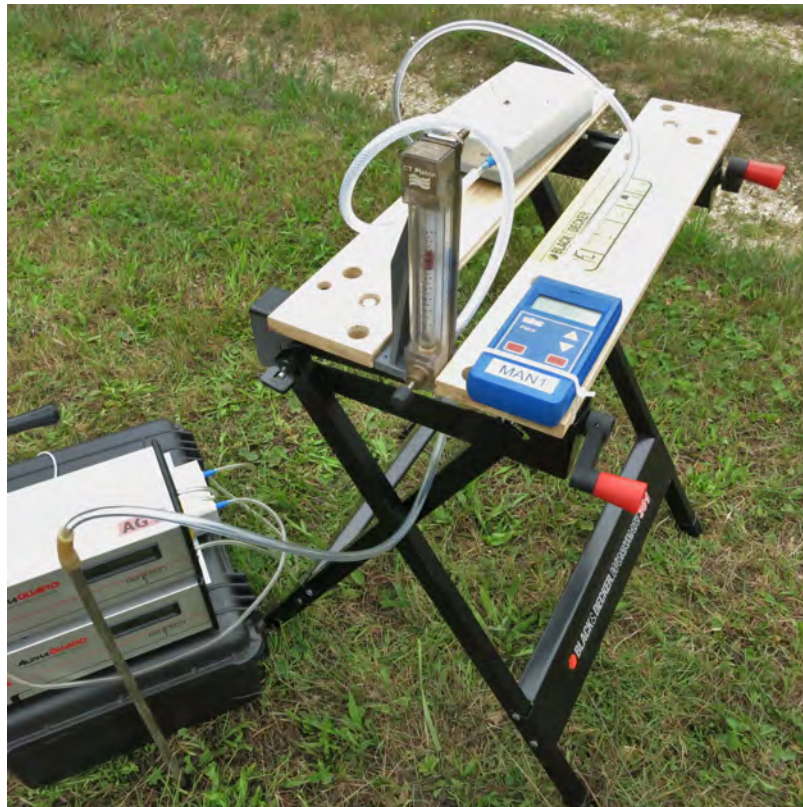
Figure 6.6.: Photograph of the setup to measure the soil permeability.
