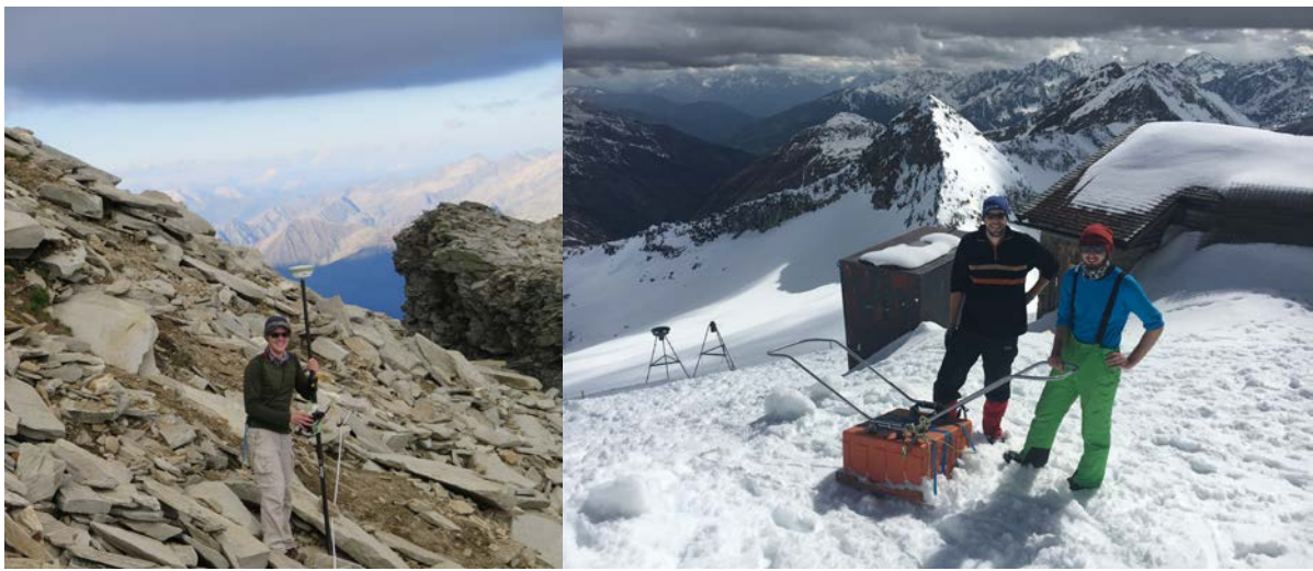
Figure 7-4: left: Establishment of a large grid with a Differential GPS (Matthias Steiner), right: profiling with 200 MHz GPR antenna (Jakob Gallistl, Raphael Vasak)
