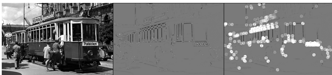
Figure 3.2: Corner detection. Left : Original image, centre : filtered image using corner detector, right : Corners (white circles) are the filter’s strongest responses.
