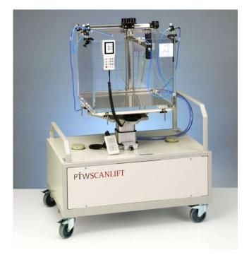
Figure 3.3: MP3-M water phantom system of PTW [PTW12]
